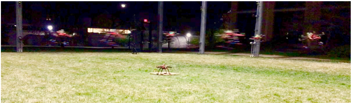
Figure 2.27: Tractor hexacopter tracking a circular trajectory with tangential velocity 2.2m/s .
