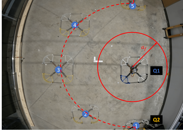
Figure 6.1: Q1 fails and stays in place within the solid red circle. Q2 uses the CEM navigation algorithm to smoothly avoid the failed vehicle and travels along the dashed red path. The blue circles indicate five time points for Q2.
