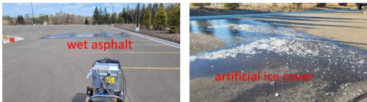
Figure 5.14. Photos of the smooth asphalt surface covered artificially by water and ice.
