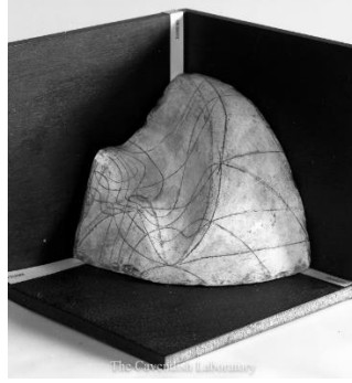
Figure 3-13: Photo (taken by Walter Andrews) of Maxwell’s model of Gibbs’s thermodynamic surface of water (1876). 167
