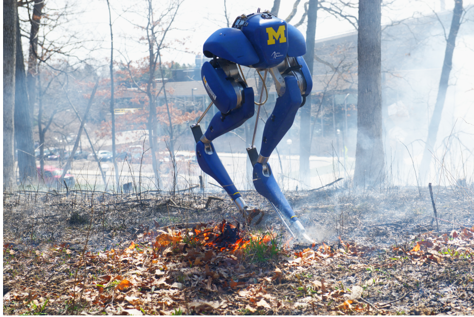
Figure 1.1: Cassie walking through burnt ground. Legged Robots have the potential to replace humans in dangerous situations. 1
