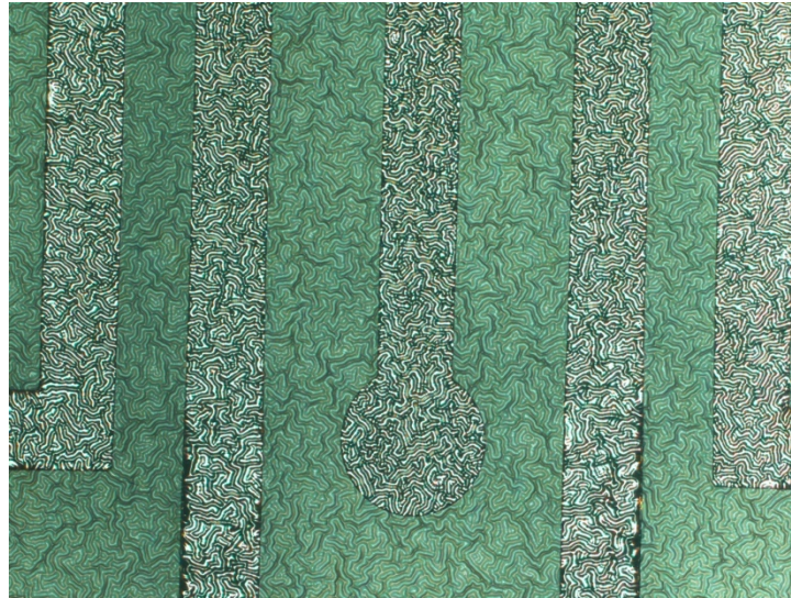
Figure 11 Cr/Au/Cr metal layer deposited on PDMS. Conductive tracks were designed to be 100\ \mu\text{m} in width and the circular electrode to be 200\ \mu\text{m} in diameter.
