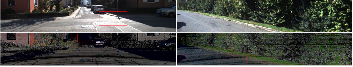
Figure 4.4: Examples of Failure modes for the proposed method. Top row are ground truth RGB images, bottom row are the corresponding lit images using the proposed method. Red squares are used to highlight specific failure modes of the proposed method. In the first column, the proposed method is unable to replicate the overexposed road in the target RGB image (highlighted by the red square in the top image; this saturation effect is absent in the predicted image below). We also see that there are artifacts introduced by the scanning geometry of the Lidar sensor. For example, we cannot light/reconstruct the parts of the scene that have no Lidar data, which is also highlighted in the first column (red square bottom image). In the second column, the beam artifacts of the Lidar scan are highlighted in the lit image.
