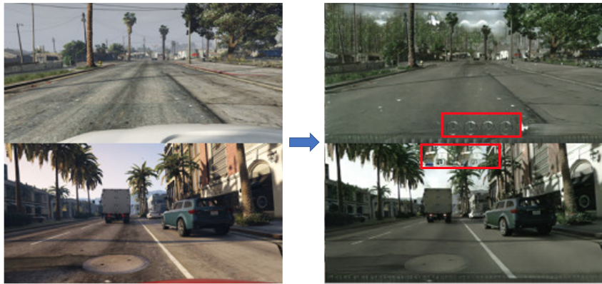
Figure 1.2: The virtual images from GTA are on the left; on the right are the corresponding images translated by CycleGAN [169] into the "real world", specifically the Cityscapes dataset [29]. The negatively transferred features are highlighted in the red boxes
