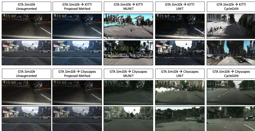
Figure 2.4: Qualitative comparison of unaugmented GTA Sim10k in the first column, Sensor Transfer augmented GTA Sim10k images in the second column, MUNIT augmented GTA Sim10k in the third column, UNIT-augmented GTA Sim10k in the fourth column, and CycleGAN-augmented GTA Sim10k in the last column. The first two rows are GTA Sim10k translated to the KITTI domain, and the second two rows are GTA Sim10k translated into the Cityscapes domain. Note that, for the Sensor Transfer augmented images, the primary sensor effect transferred in GTA Sim10k → Cityscapes augmentation is decreased exposure, whereas the primary sensor effects transferred in GTA Sim10k → KITTI augmentation is a blueish hue and increased exposure. In comparison, images augmented using the image-to-image translation networks lose a significant amount of spatial information. These methods also cannot handle night time images as well as the proposed method.
