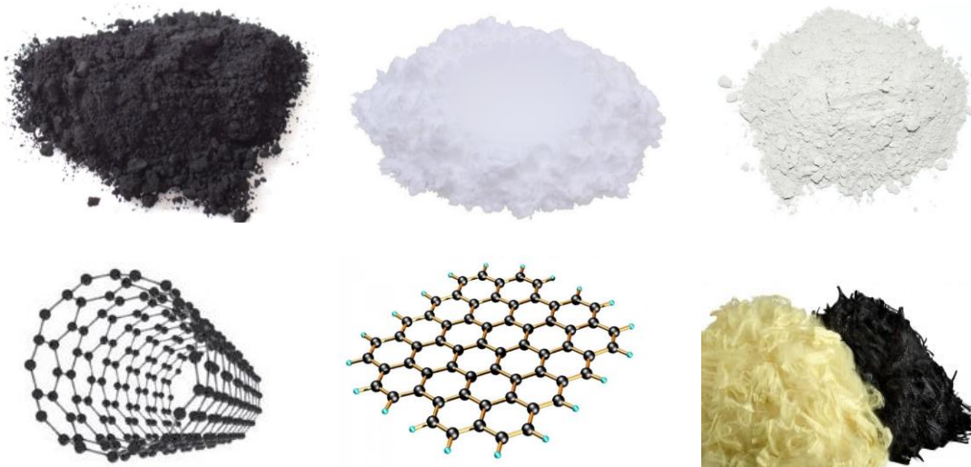
Figure 1.7. Reinforcing fillers: carbon black, silica, nano clays, CNTs, GOs, and short fibers (from upper left to right).
