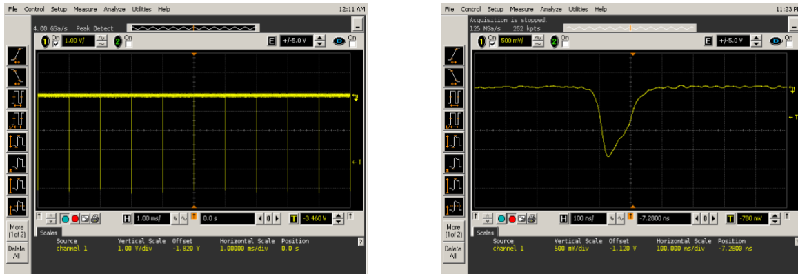
Figure 4. 2: Screen shot of (a) 1kHz pulse train (b) pulse duration
