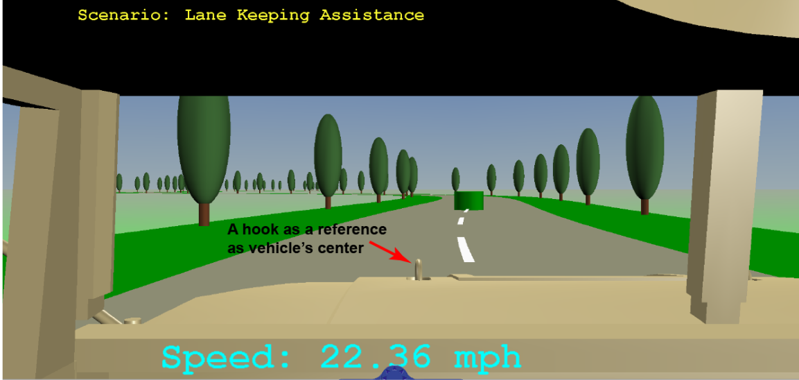
Figure 2.3: Visualization module based on Simulink 3D Animation Toolbox. The highlighted hook is a reference for the subject to find the center of the vehicle.
