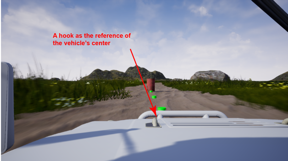
Figure 2.4: Visualization module based on Unreal Engine 4. The highlighted hook is a reference for the subject to find the center of the vehicle.
