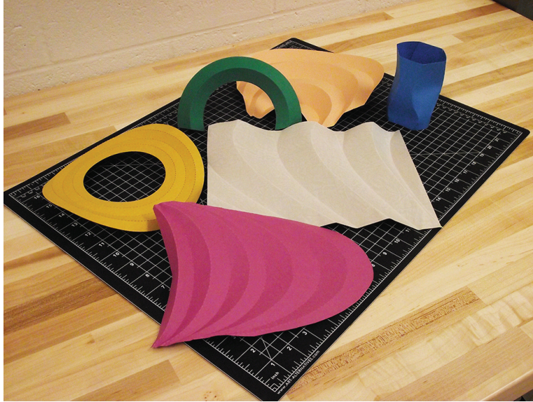
Figure 1.1 – Paper models of folded curved-crease origami geometries.
