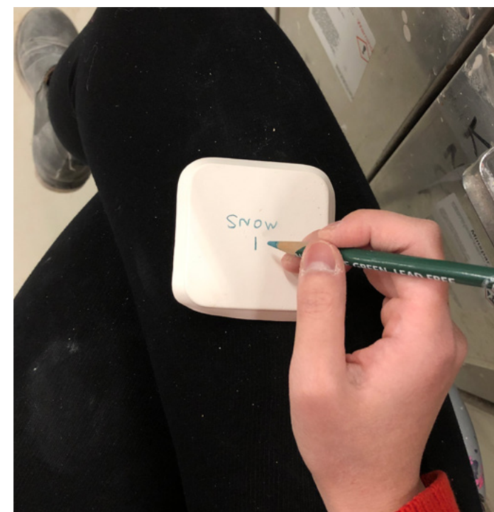
Labelling test tiles with their corresponding base glaze and colourant addition code
