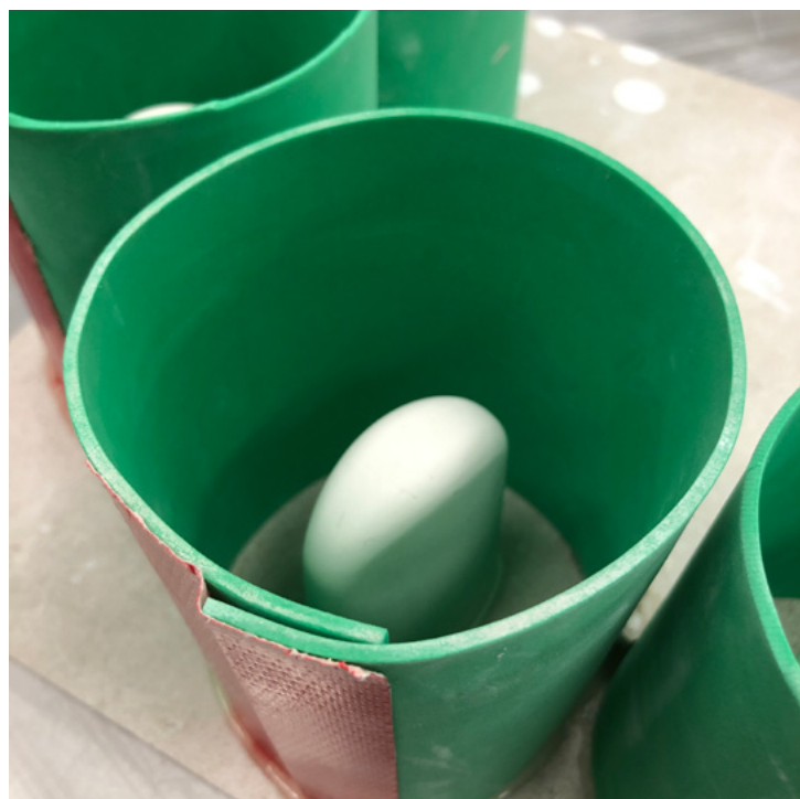
Making plaster moulds for slip-casting test tiles using a positive model made from store-bought popsicle mould
