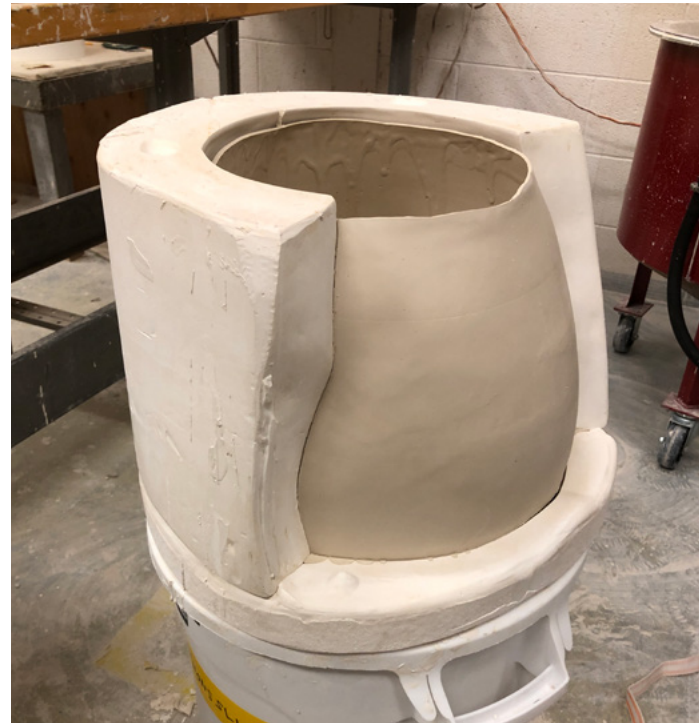
Demoulding slip cast from the mould after it has dried to leather hard
