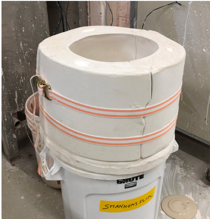
Four-part mould prepared for slip casting
