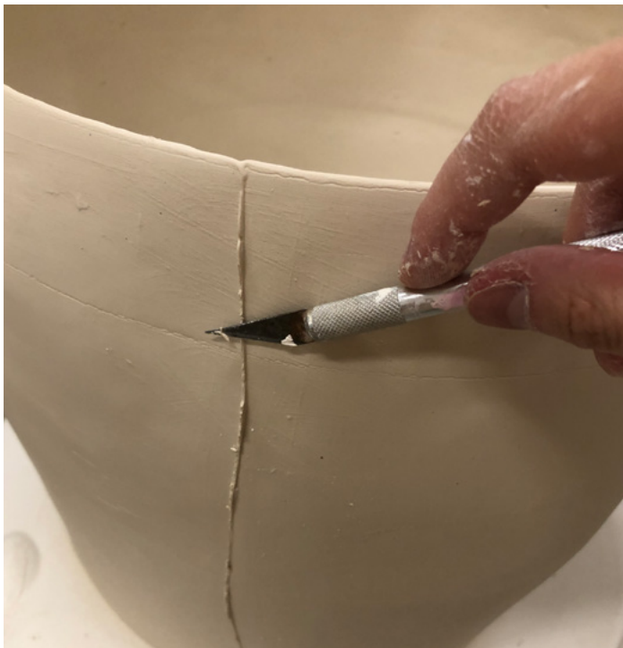
Trimming excess clay at the seams of where the mould parts meet
