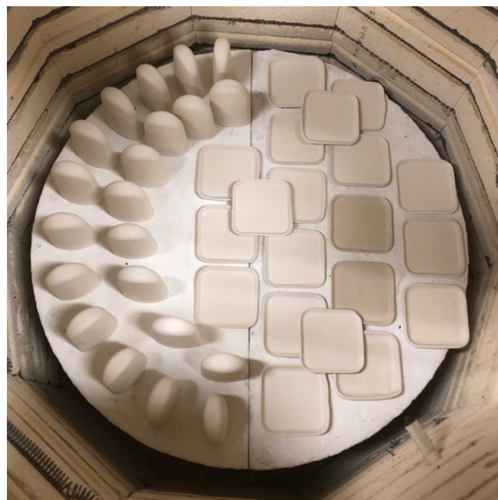
Firing test tiles (left) and catchers (right) to bisque temperature
