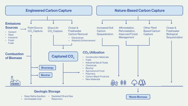
Figure 16 Recommended prime solutions for carbon offset projects in the Great Lakes region. Each type of solution shown above was evaluated based upon different metrics listed below such as cost, land use, water consumption, risk of reversal, and implement readiness. Source: Adapted by authors from the CDR Primer.
