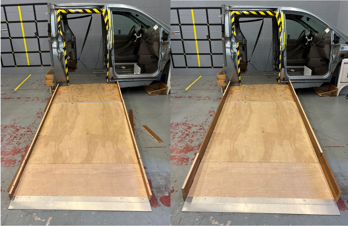
Figure 2. Baseline low edge guard C (left) and high edge guard D (right) ramp conditions.
