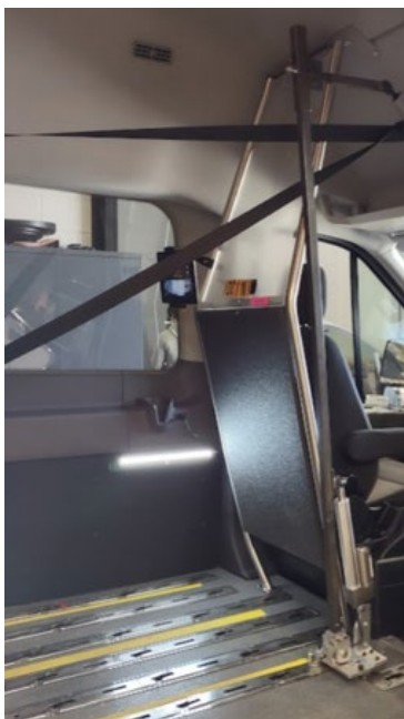
Figure 7. Automated donning arm used in Condition A.
