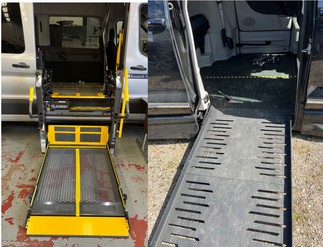
Figure 1. Lift in condition A (left and ramp in condition B (right)).
