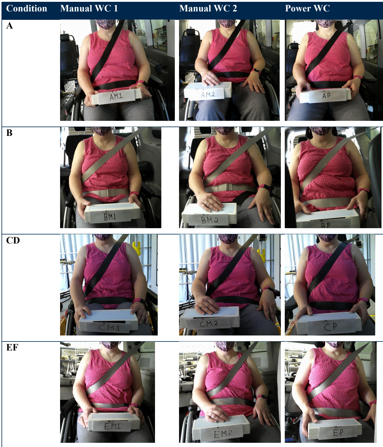
Figure 8. Example belt fit across vehicles and wheelchairs for exemplar person.
