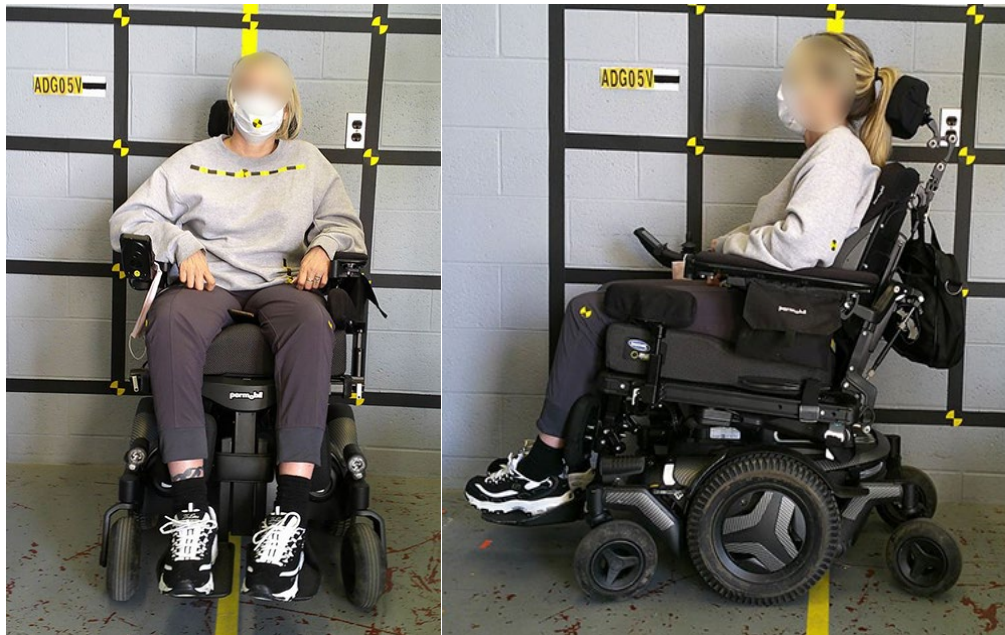
Figure 13. Examples of reference photos to estimate dimensions and posture of person and their wheelchair.
