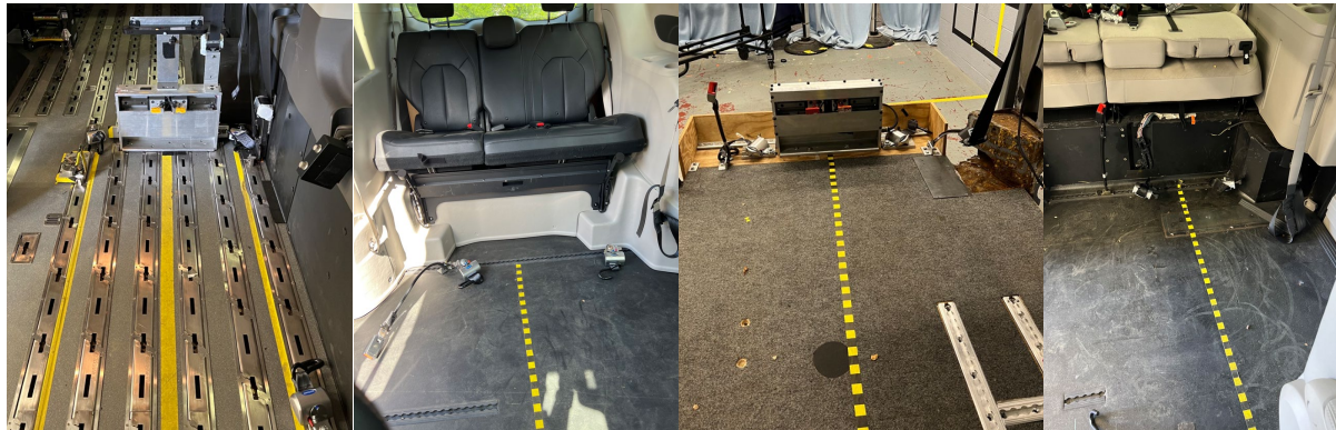
Figure 6. Wheelchair station, docking, and lap belt hardware for Configuration A (left), B, (left center), CD (right center) and EF (right.)
