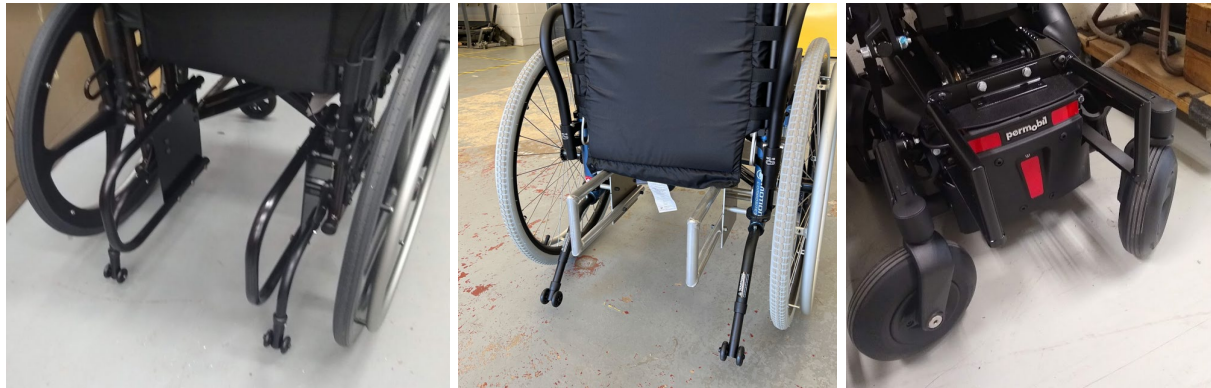
Figure 12. Manual wheelchair 1, a Sunrise Quickie 2 (left), Manual wheelchair 2, a Helio (center), Power wheelchair, a Permobil F3 Corpus (right), each equipped with custom UDIG-compatible attachments.
