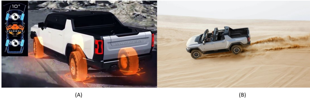
Figure 3: 2022 Electric Hummer: Drive mode — (A) Crab mode; (B) Baja mode
