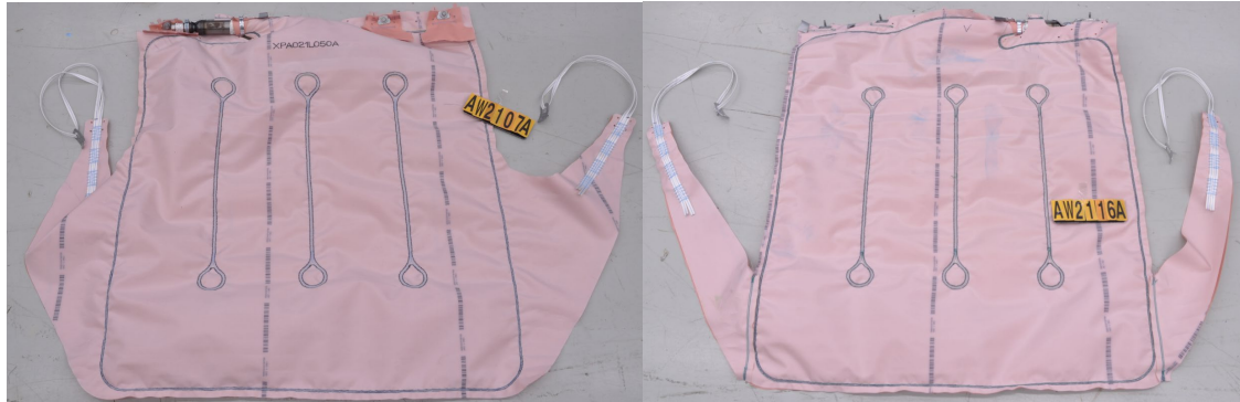
Figure 126. CATCH-V (left) with original tether design and CATCH-V' (right) with alternative tether design.
