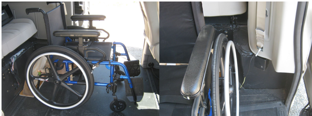
Figure 88. Manual wheelchair and UDIG anchorages in Braun vehicle; lateral location limited by wheel well.
