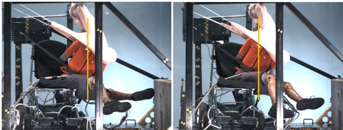
Figure 125. Front view at time of peak excursion for test AW2107 (left) and AW2109 (right), showing reduced lateral excursion with tether location 2.
