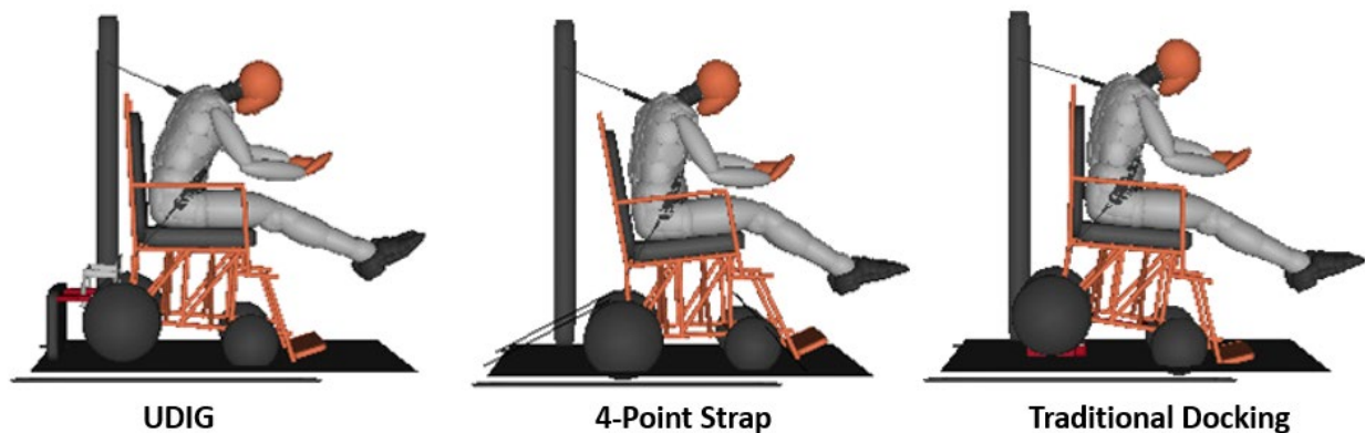
Figure 139. Comparison of peak forward excursion in frontal crash simulations with UDIG, 4-point strap tiedown and traditional docking.
