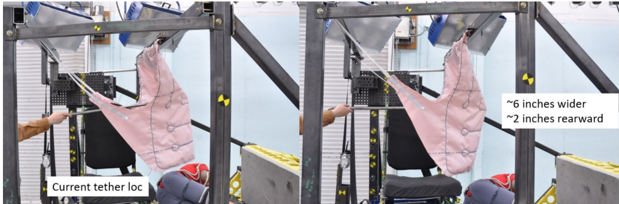
Figure 124. Static photos of sled buck showing location of CATCH bag when tethers reach the point of no slack with tether location 1 (left) and tether location 2 (right).
