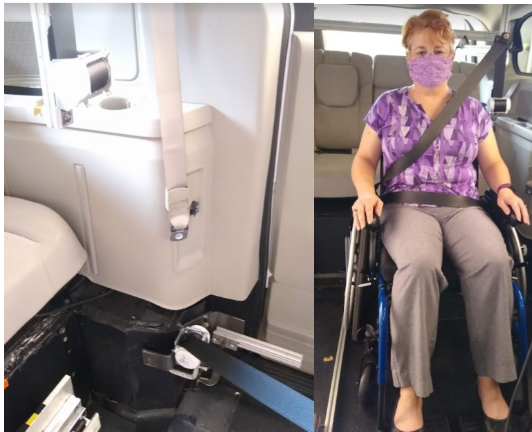
Figure 153. Seatbelt with dual retractors installed (left) and providing snug belt tension on pilot volunteer (right).
