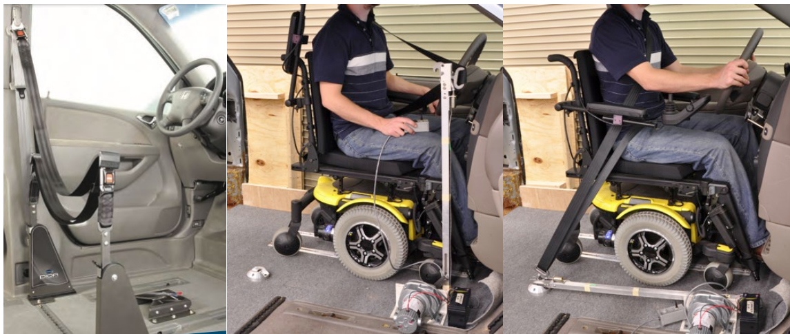
Figure 10. Q'Straint DIOR self-donning belt system top) and UMTRI prototype belt donning system (lower left and right).
