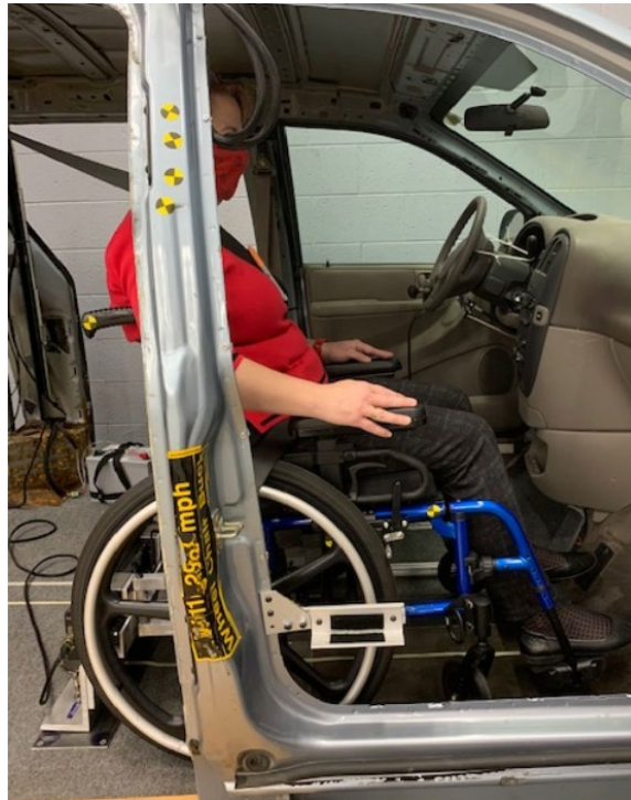
Figure 93. For current vehicle configurations, a right-front position that allows the required 122 cm (48 in) long space for a wheelchair places the UDIG well behind the B-pillar.
