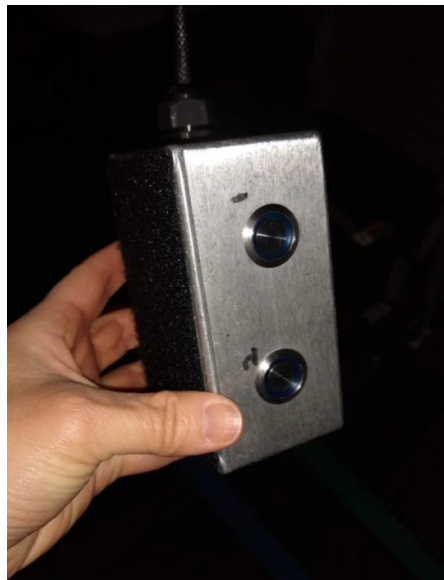
Figure 114. Photo of actuator controls.
