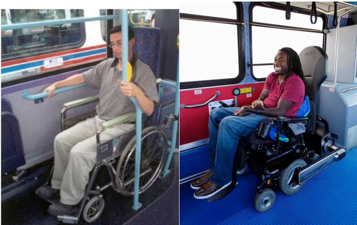
Figure 3. Rear-facing wheelchair passenger station (left) and Q'Straint Quantum automated docking system (right).
