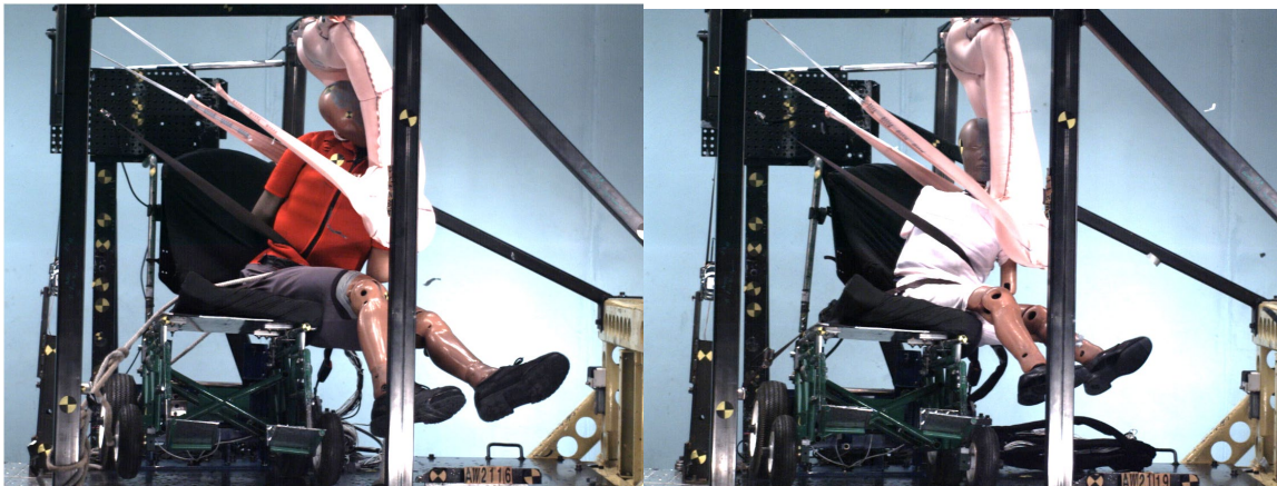
Figure 134. Peak excursion between ES2-RE (left) and SID-IIS (right) using CATCH-V' and SWCB.
