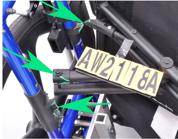
Figure 133. Damage to manual wheelchair during test AW2118.
