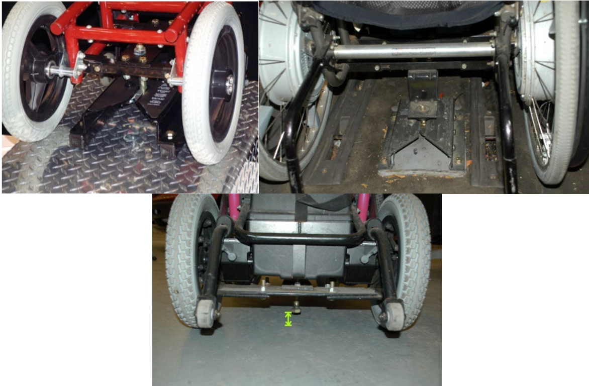
Figure 1. Examples of wheelchairs engaged with docking systems mounted to vehicle floor (upper left and right) and example of mating hardware with low ground clearance (lower center).
