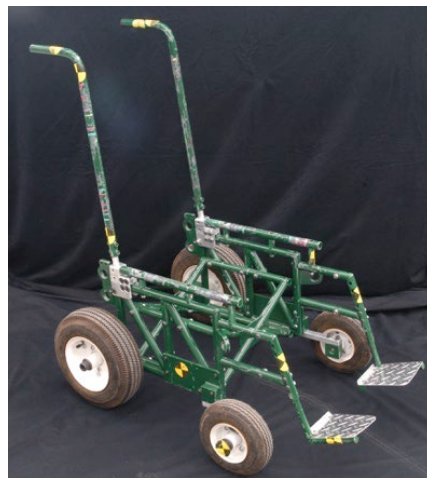
Figure 14. Surrogate wheelchair and surrogate wheelchair frame.
