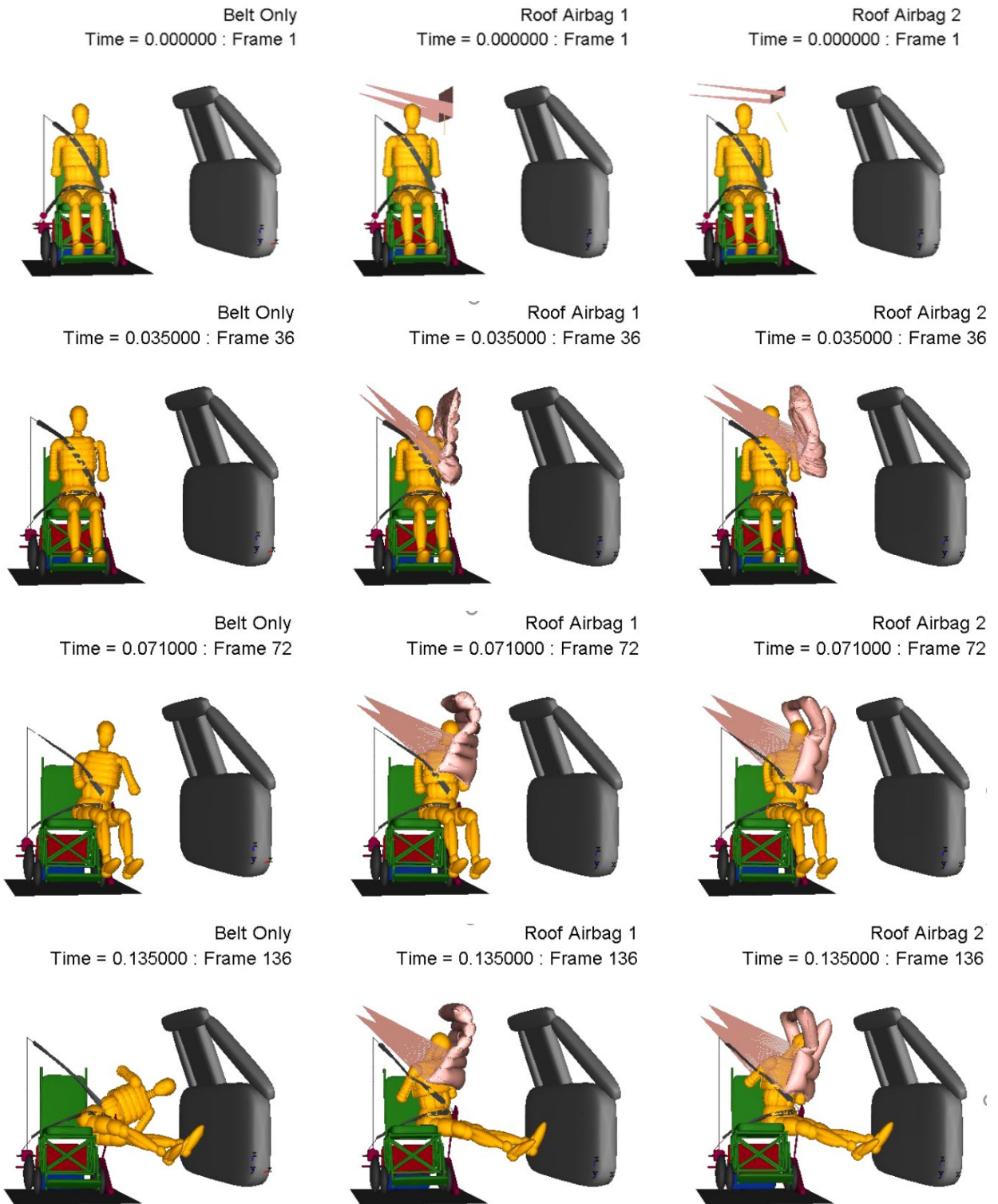
Figure 56. Comparison of kinematics in farside impact for belt only (left), CATCH 1 design (middle), and CATCH 2 design (right).
