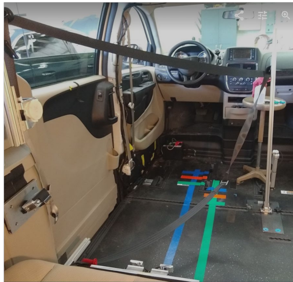
Figure 90. Duct tape used to mark centerlines and space 123, 137, and 152 cm (48, 54, and 60 in) forward of the UDIG anchorages.
