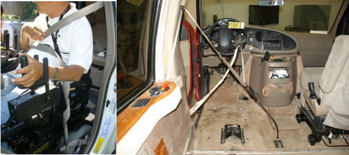
Figure 7. Driver using vehicle belt with poor fit (left) and a “drive-in” belt arrangement (right).
