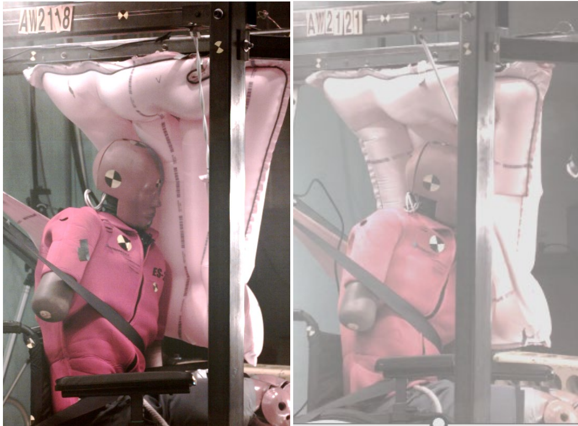
Figure 145. Comparison of head contact points in manual chair in original and shifted locations.
