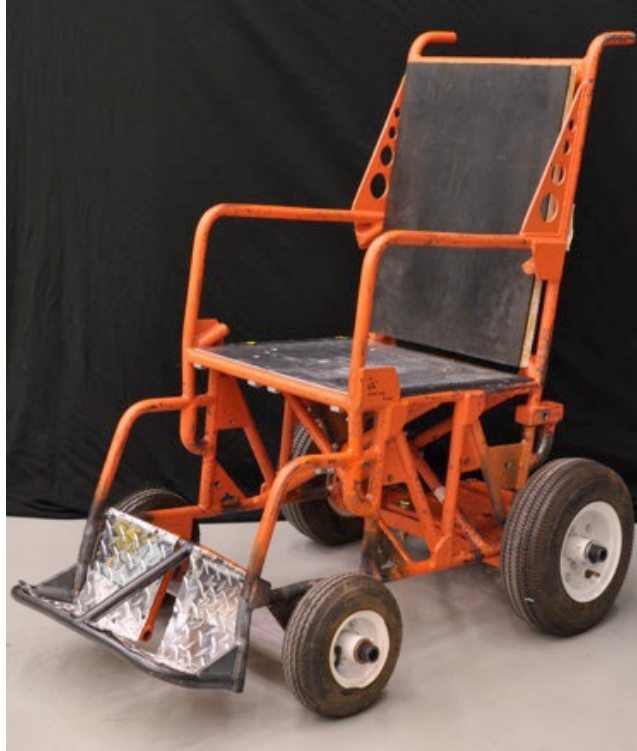
Figure 11. Surrogate wheelchair fixture.
