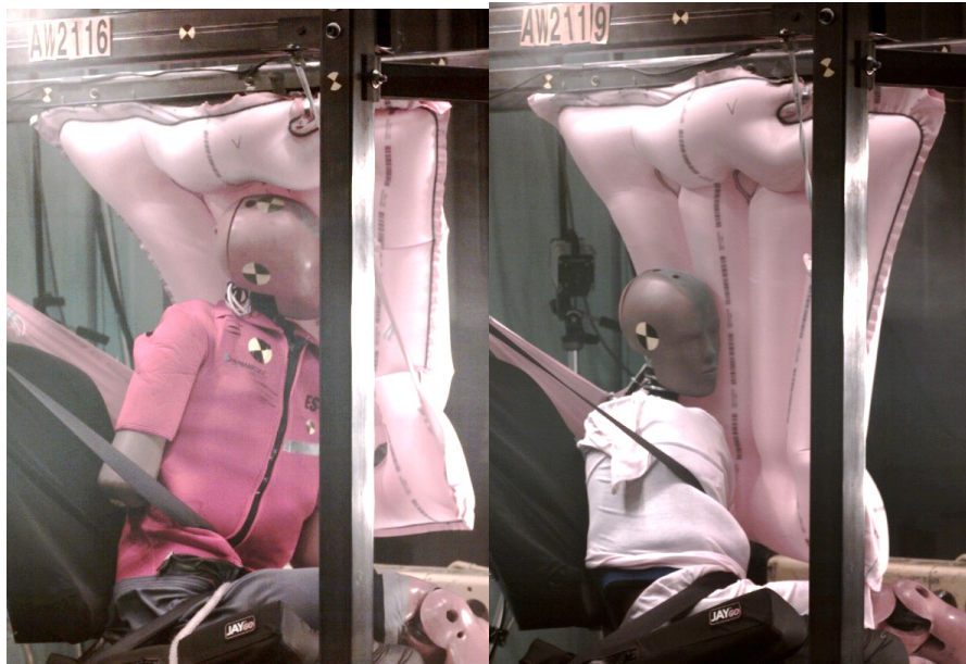
Figure 135. Peak excursion between ES2-RE (left) and SID-IIS (right) using CATCH-V' and SWCB.
