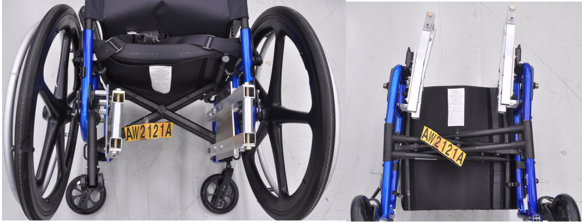
Figure 146. Deformation to UDIG attachments during side impact in AW2121. Rear view (left), bottom view (right).
