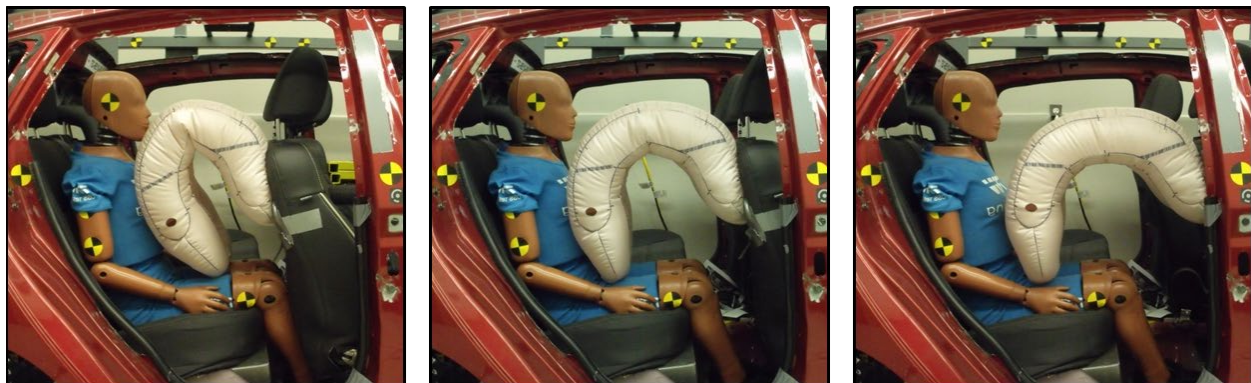
Figure 29. SCaRAB Design adapting to varied occupant space
