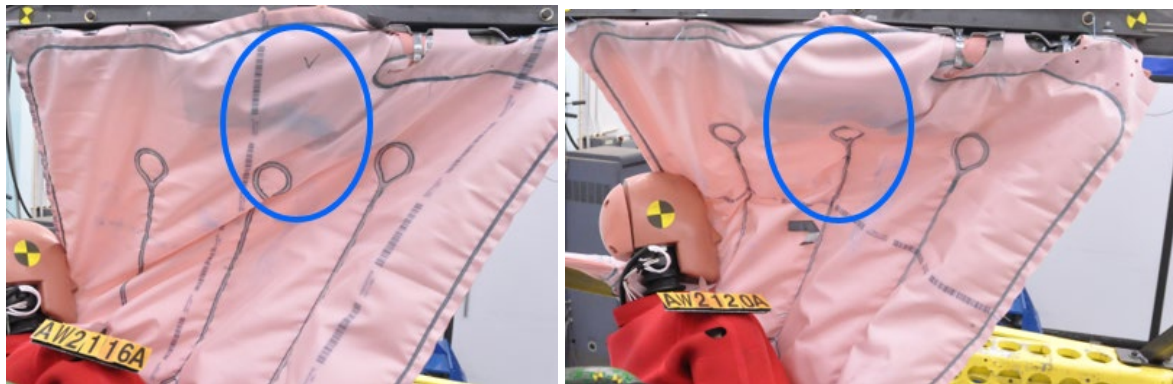
Figure 143. Comparison of head contact location between AW2116 change test comparison (left) and AW2120 (right).
