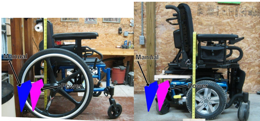
Figure 83. Overlap of optimal lap belt anchor zones for sample power and manual wheelchairs.
