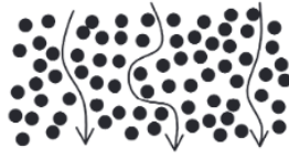
Figure 2.5: Resin percolation around fibers [2].
