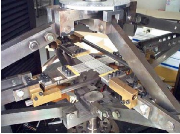
Figure 2.13: Biaxial tension test device and measuring results for different ratios [15].
