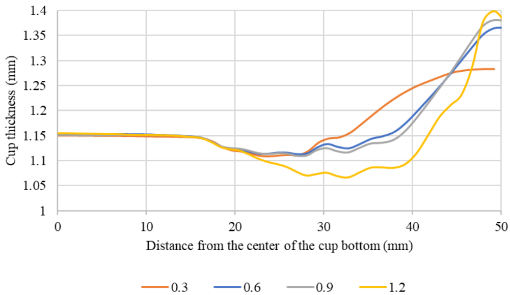
Figure 3.50: Cup thickness variation just before failure for deep drawing at different failure strain values.
