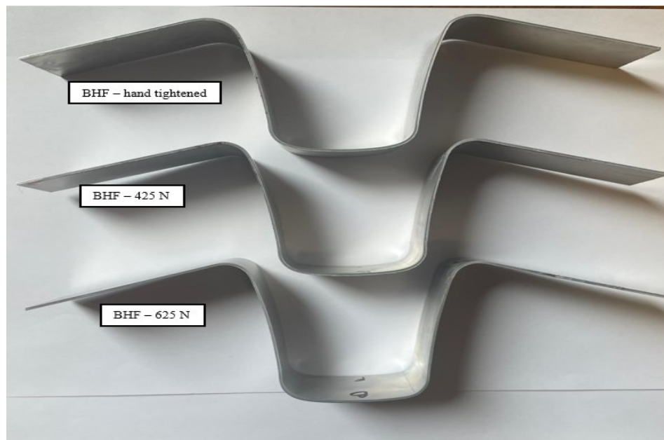
Figure 4.54: Profiles of Al/PP/Al specimens with 0.2/0.8/0.2 mm thickness combination after springback
