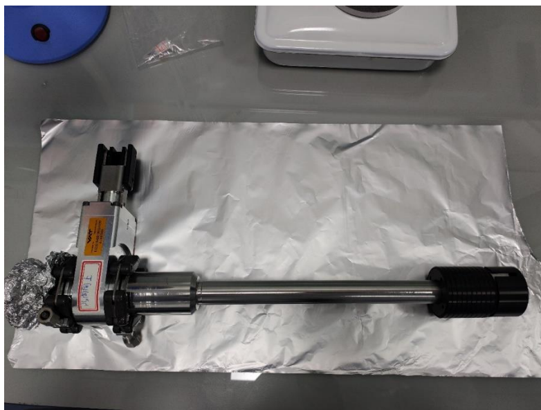
Figure S7 Photographs of the gastight container for XPS measurements.
