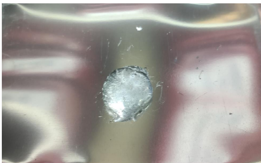
Figure S2 Photograph of the molten lithium foil in the glovebox.
