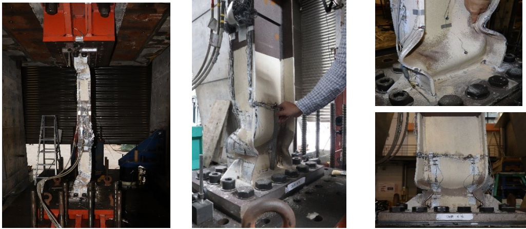
Figure 14 Observed performance of IC-49-I (0.04 rad drift)
