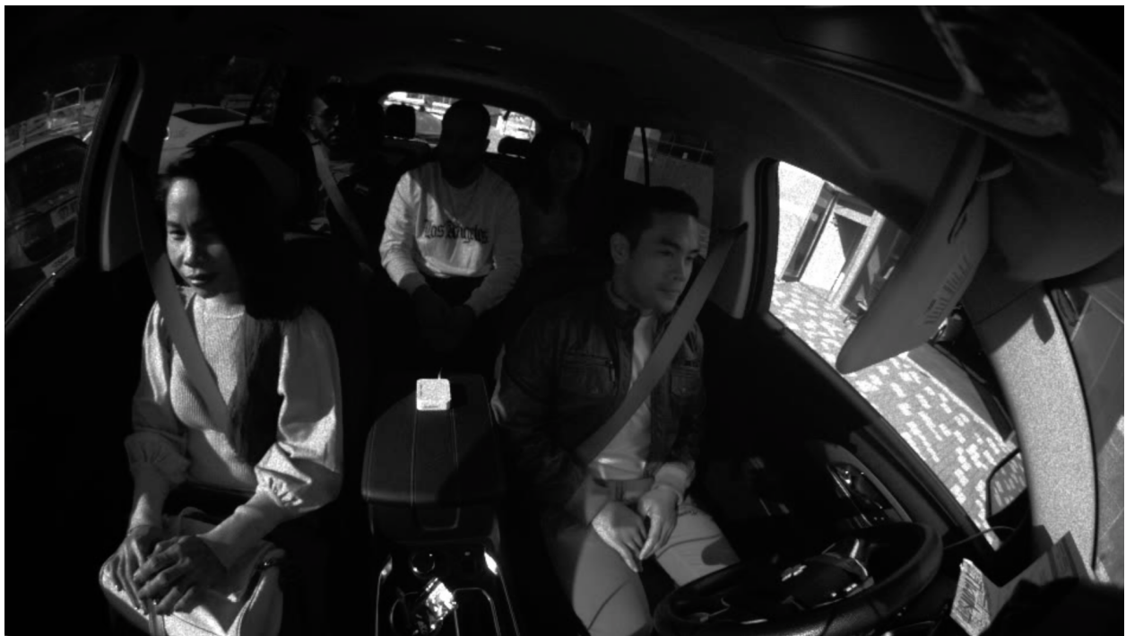
Figure 8.3: Occupant-monitoring RGB-IR perspective sample. This camera technology is more sensitive to ambient light and generally harder to see the illumination.
