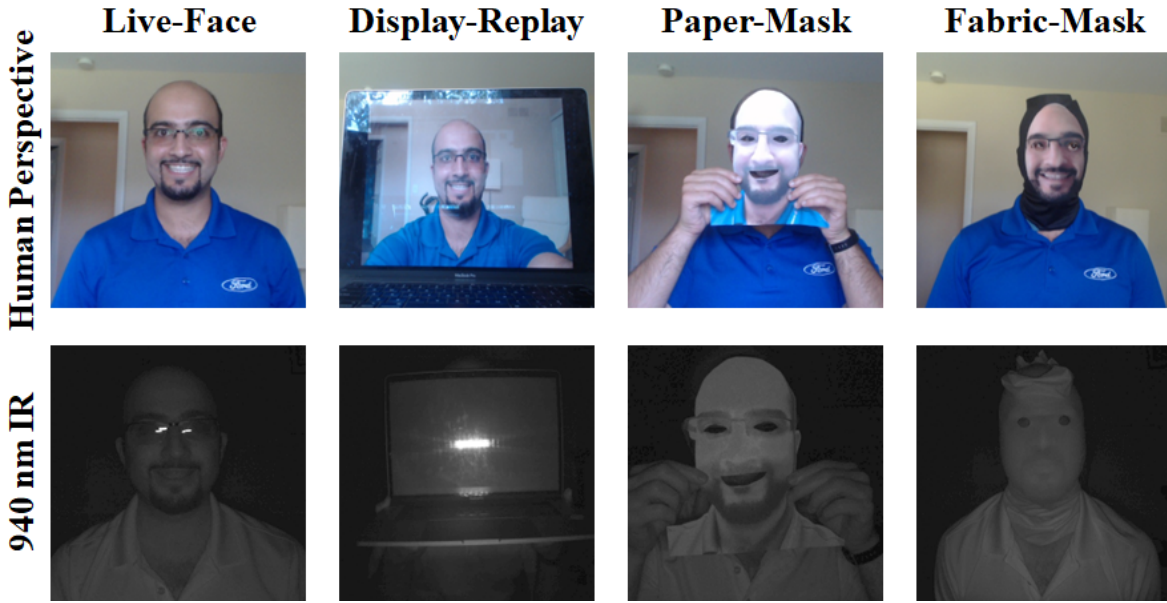
Figure 6.1: Juxtaposing the human and illuminated near-infrared perspectives. Note how illuminated near-infrared yields distinct reflectance-patterns. Live faces have complex texture; spoofs conversely appear washed out.
