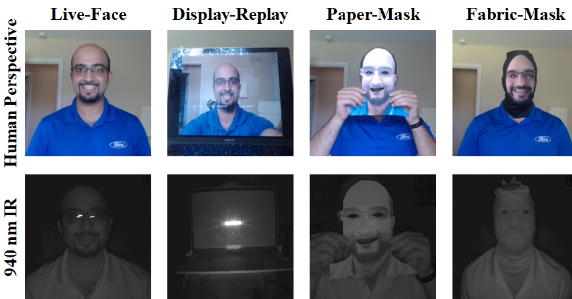
Figure 4.1: Juxtaposing human and illuminated near-infrared perspectives. Spoofs have less texture variance and appear brighter to the infrared camera.
