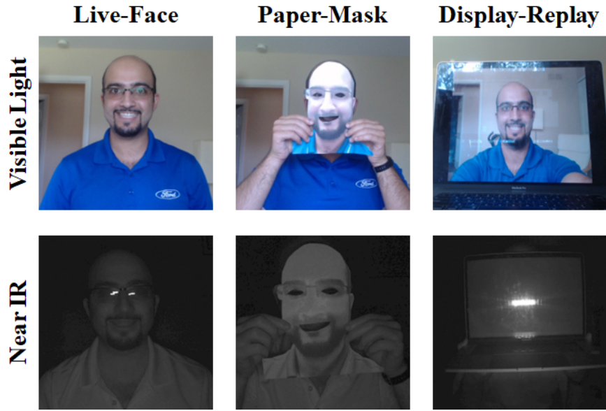
Figure 5.1: Visualizing common spoofs in RGB versus NIR. Presentations in order: live-person, paper-mask and display-replay.
