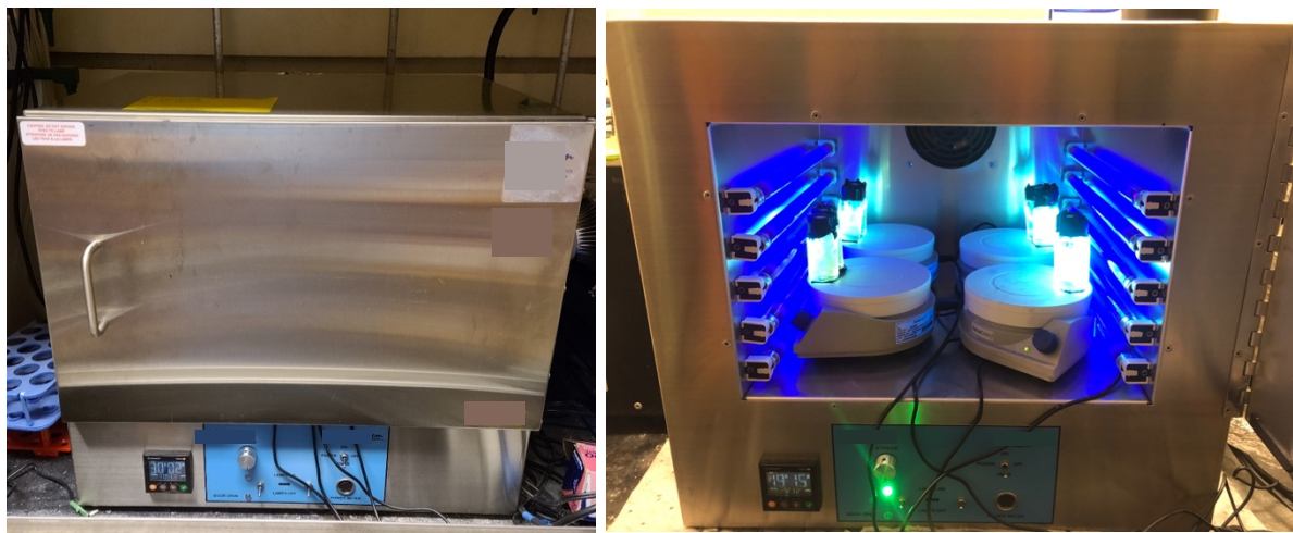
Figure S1. The photochemical setup used in this study shown with the door closed (left) and the lights on/door open (right). These photographs were taken in the Sanford Laboratory by Matthew R. Lasky.
