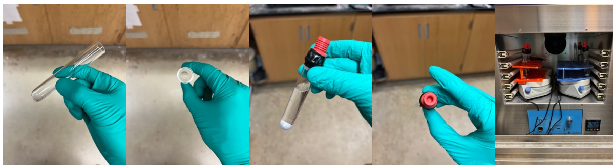
Figure S2. Quartz test tubes utilized when irradiating with UVB CFLs. The photochemical setup employed for the quartz tubes is depicted on the far right. These photographs were taken in the Sanford Laboratory by Matthew R. Lasky.
