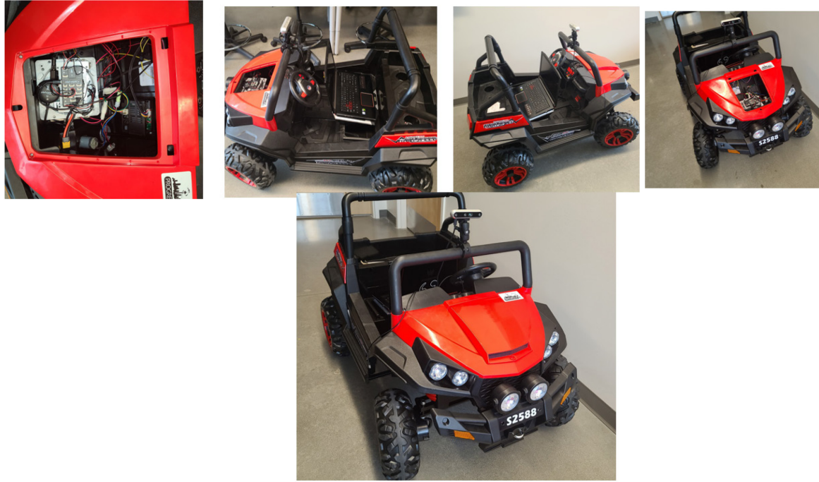
Figure 4-4: The OSCAR_PX4 system plugin with EFI V Twin High-Speed Ride-On Car.
