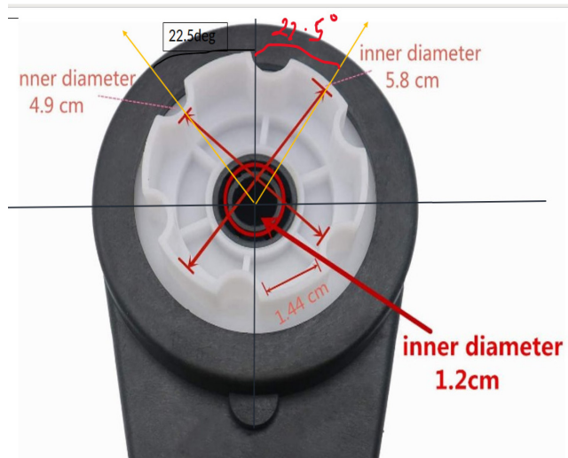
Figure 5-13: Maximum angle measurement from the vehicle motor and steering column.
