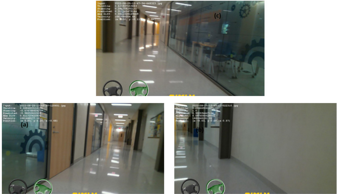
Figure 8-4: The vehicle performance during neural network testing. (a) A screenshot of the Visualization interface turning right for actual and predicted data. (b) A screenshot of the Visualization interface turning left for actual data and predicted data. (c) A screenshot of the Visualization interface moving straight for actual and predicted data.
