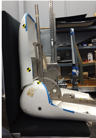
Figure 10. SAE J826 H-point machine in test seat (weights not shown).
