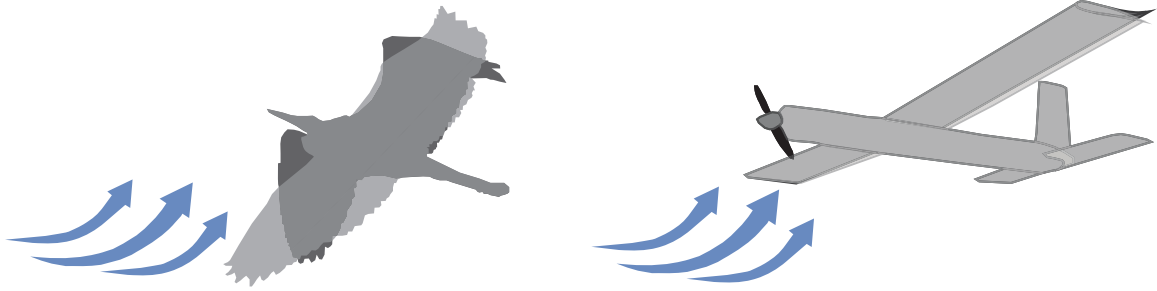
Figure 4.1: Birds change the shape of their wings to react to environmental changes. This inspired the use of camber morphing to create smooth shape changes that adjust lift production in response to gusts.
