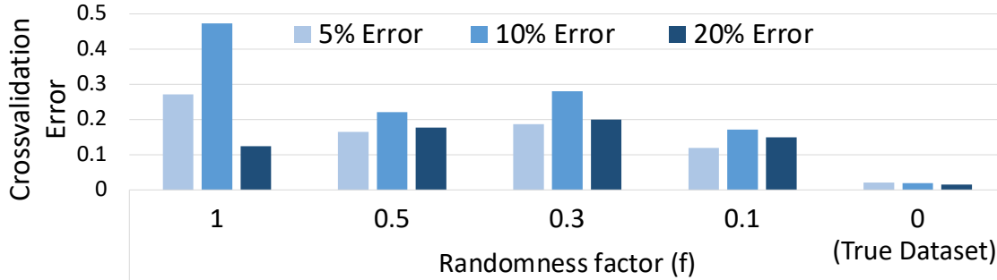
Figure 3.6: Cross-validation errors of decision trees trained for the video camera over a range of error tolerance limits.
