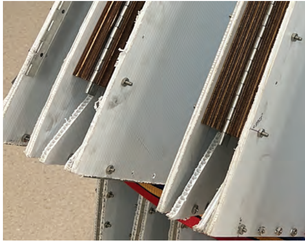
Figure 5.2: The zoom-in view of a meter-scale origami tube assembled by connecting corrugated panels with piano hinges (tube courtesy: Anna Jia and Yi Zhu).
