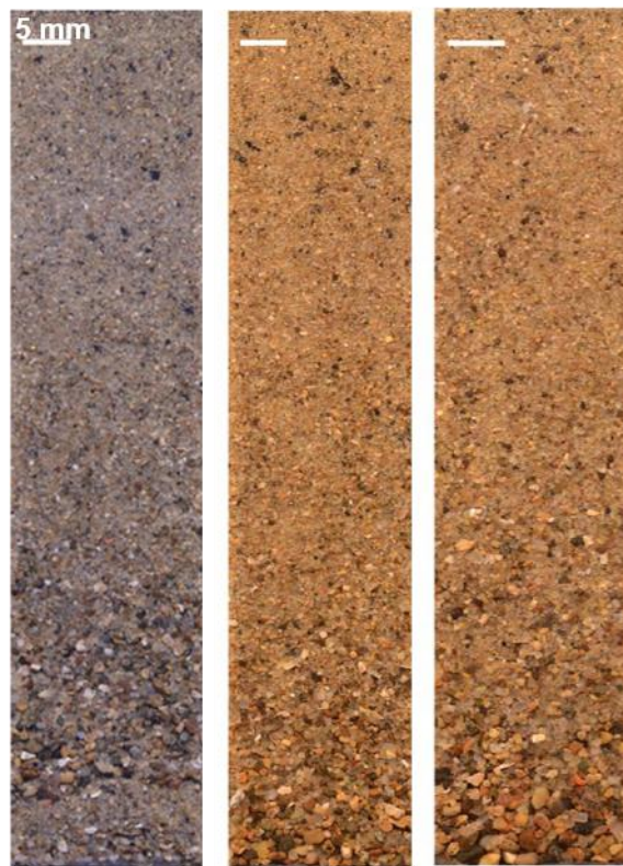
Figure 3-15. Specimen C. (Top) verification PSDs, (Bottom) Field [left], Field-Repeat [center], and Lab [right] photographed FieldSed sides.
