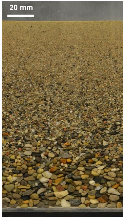
Figure 3-26. Unwrapped cylinder image of example sand tested with the Sed360 system.
