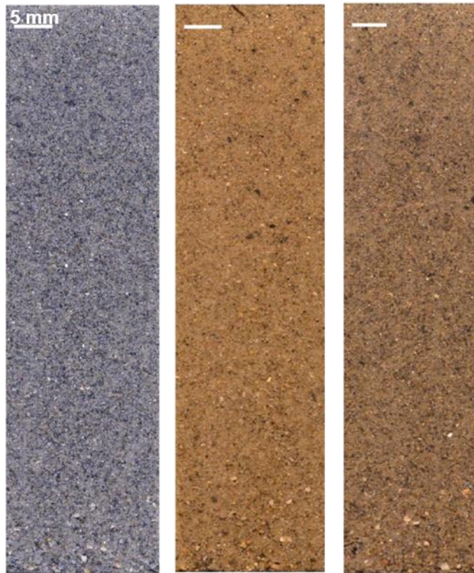
Figure 3-18. Specimen F. (Top) verification PSDs, (Bottom) Field [left], Field-Repeat [center], and Lab [right] photographed FieldSed sides.
