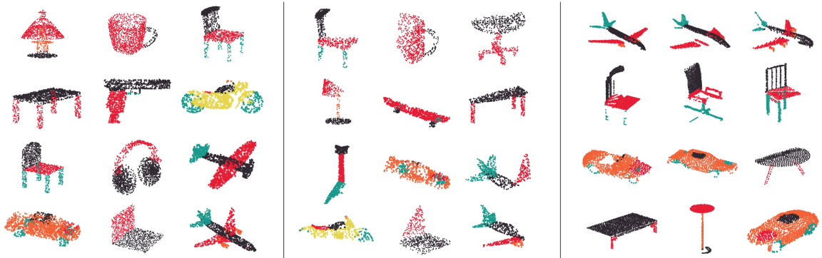
Figure 4.4: Qualitative results on part segmentation of point clouds using the method presented in this work. Different colors correspond to distinct segments. Left: segmentation on the ShapeNet part dataset. Middle: segmentation on the simulated partial point clouds in the ShapeNet. Right: segmentation on the Completion3D dataset.
