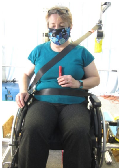
Figure 16. Belt fit of pilot volunteer in wheelchair with baseline geometry as donned; belt is caught on rear armrest.
