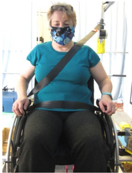
Figure 17. Belt fit of pilot volunteer in wheelchair with baseline geometry, adjusted to improve fit.
