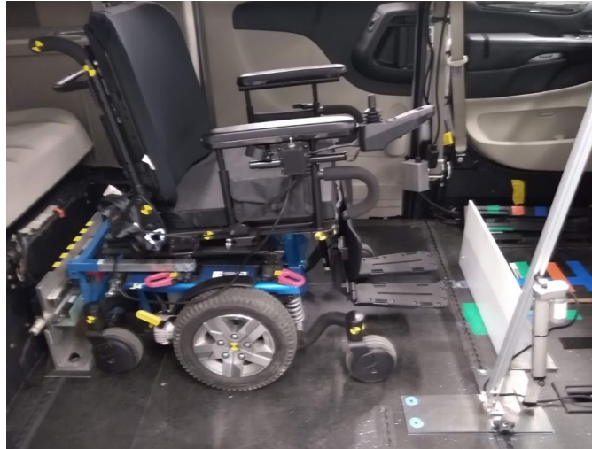
Figure 12. Illustration of barrier to restrict space in Braun van.
