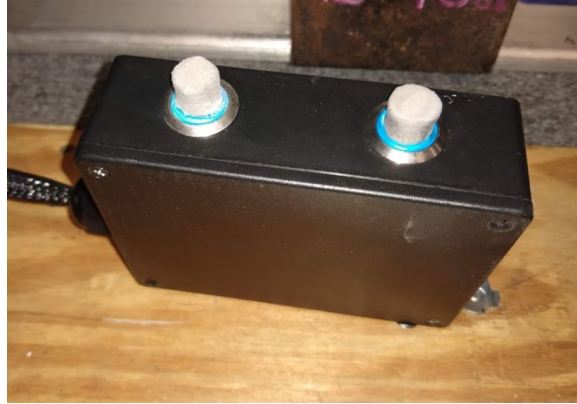
Figure 19. Revised control buttons for people with limited dexterity.
