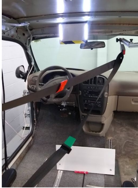
Figure 14. LED panel lights up on each side when UDIG hooks are engaged, plus barrier to restrict forward space.
