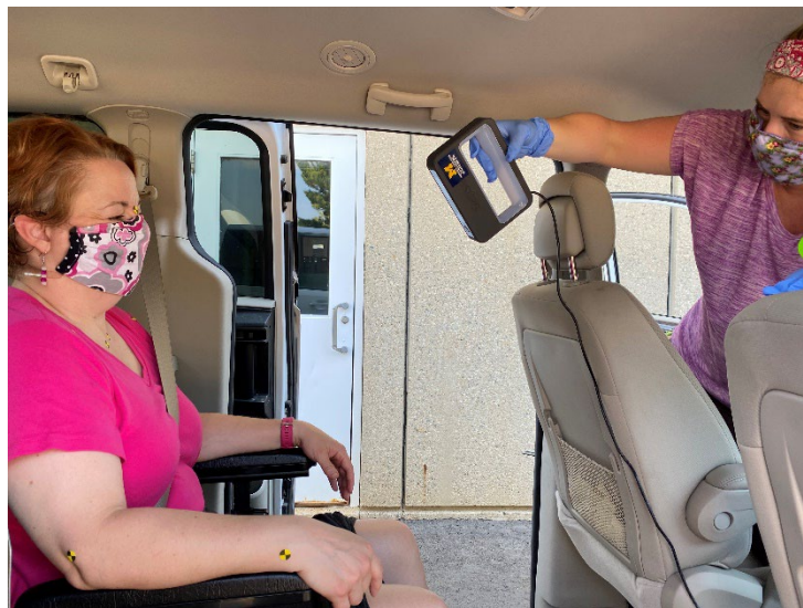
Figure 7. Measuring volunteer belt fit with remote scanner instead of FARO arm.
