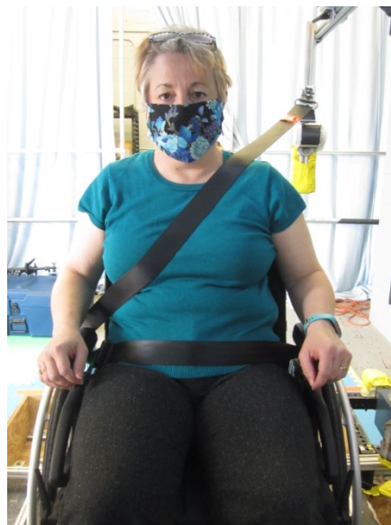
Figure 18. Belt fit of pilot volunteer in wheelchair with belt geometry adjusted to provide better fit.
