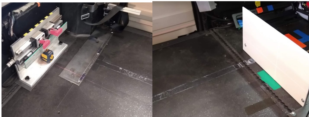
Figure 13. Replaced duct tape centerlines with a laser that shows alignment centerline on floor and cross on barrier.
