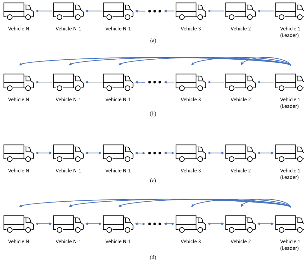
Figure 3-2. Common leader-follower communication topologies, adapted from [77]: (a) predecessor following; (b) predecessor-leader following; (c) bidirectional; (d) bidirectional-leader.
