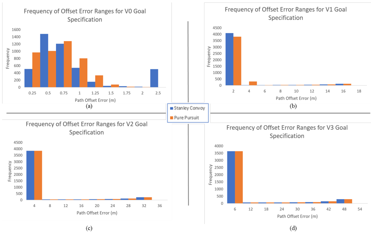
Figure 2-10. Histograms of path following error for Requirement 1 for (a) Vehicle 0, (b) Vehicle 1, (c) Vehicle 2, and (d) Vehicle 3.
