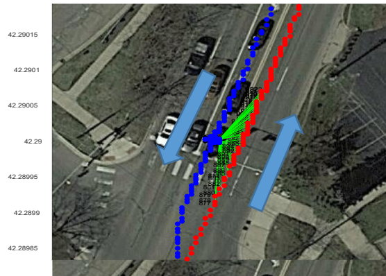
Figure 28. An example shows the relative positions between a host and a remote vehicle in one trip segment. The positions of the host vehicle are in red, and those of the remote vehicle are in blue. Two vehicles traveled in the directions indicated by the blue arrows.
