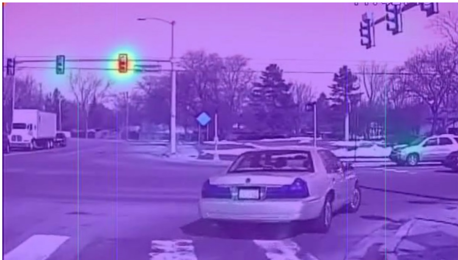
Figure 14. A heat map generated from a video frame while target vehicle was making a right-turn maneuver. Most vehicles make turn maneuver at intersections and the highlighted traffic light a crucial clue for system to determine if it's an intersection scene.
