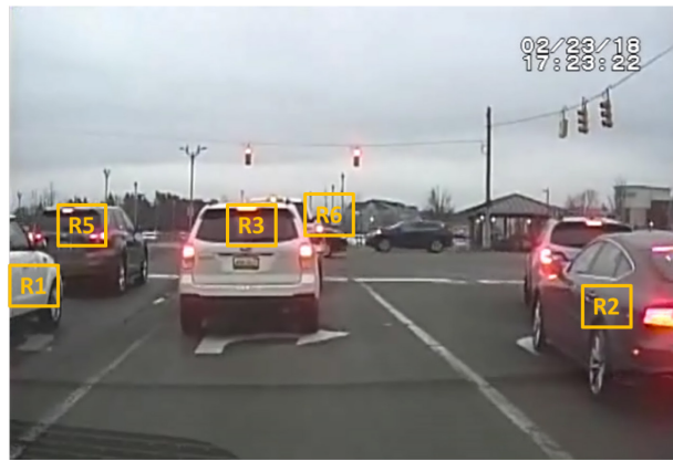
Figure 20. (a) A host vehicle H and multiple remote vehicles, R1 ~ R6 are in communication. (b) Remote vehicles seen by the host vehicle.
