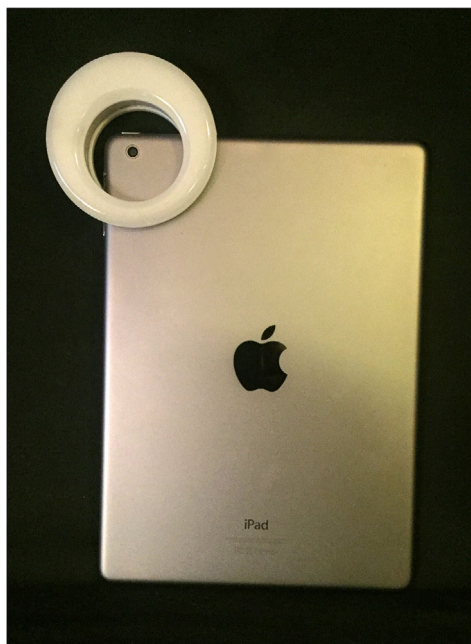
FIGURE 2 The simple supplemental ring light for use with an iPad to record videos.
