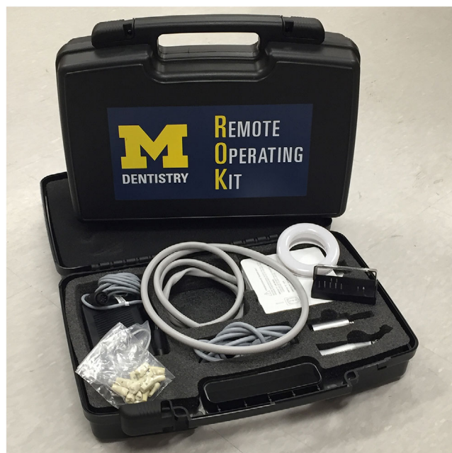
FIGURE 1 The portable case for the remote operating kit (ROK) included the handpiece motor and attachments, supplemental light for the iPad, bur block and diamonds, and replacement typodont teeth for the virtual clinic exercises.
