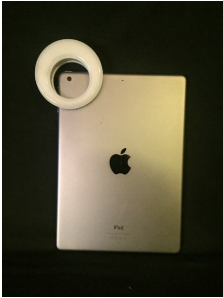
Figure 2: The simple supplemental ring light for use with iPad to record videos
