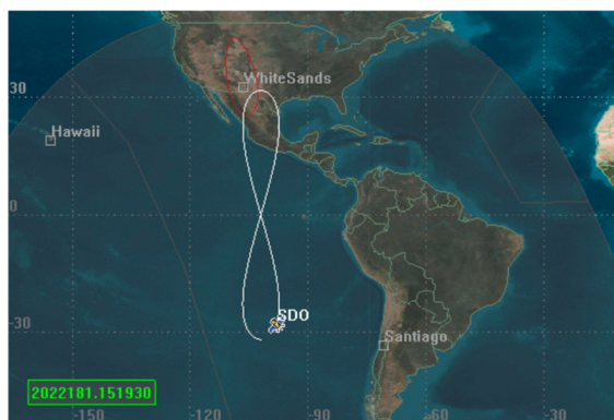
(a) The elongated figure-eight orbit as it is viewed by SDO's ground station.
