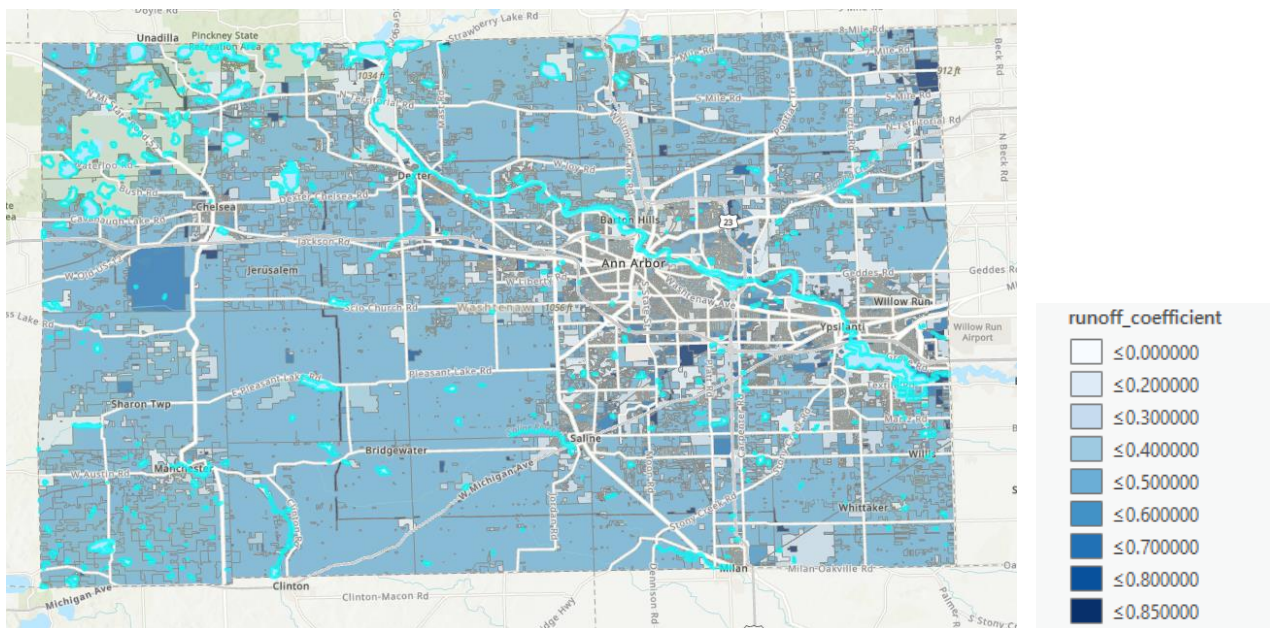
Fig. 3: Washtenaw County's various land-use types from Fig. 2 assigned their corresponding runoff coefficient values 2,3 for the Rational Method.
