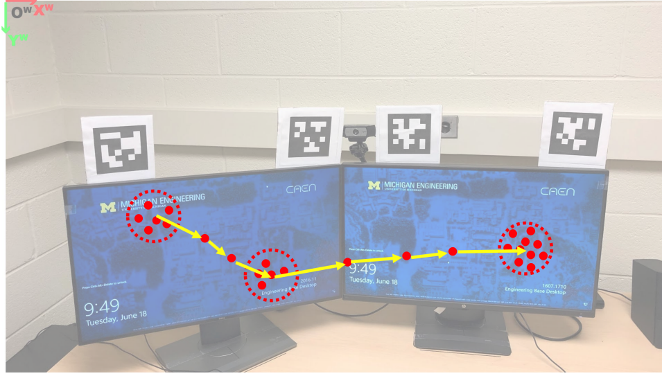
Figure 7. Illustration of fixations and saccades mapped on the world image. Red dots are gaze points. Red dashed circles are fixations. Yellow arrows are saccades.
