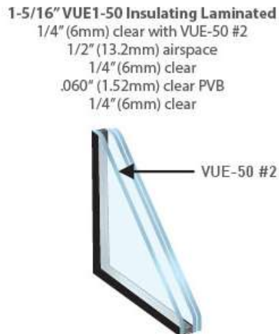
Figure 3: Dana building Skylight Laminated Glass
