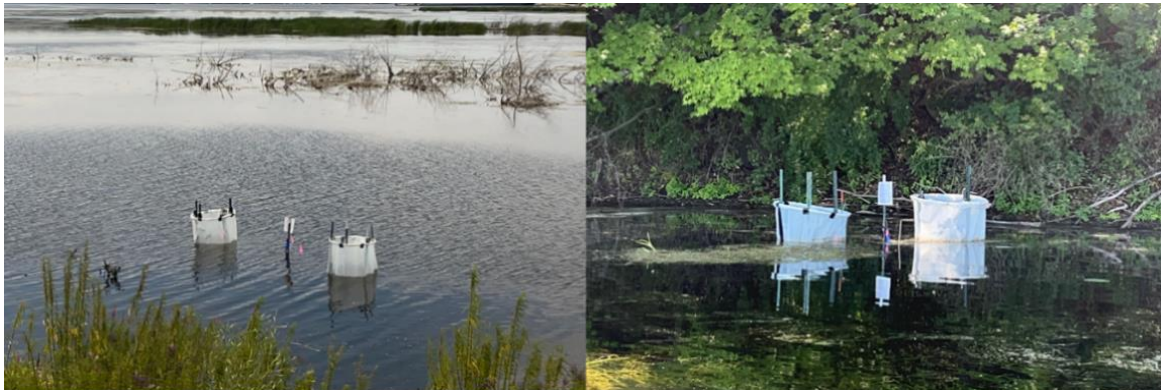
Figure 3: Limmocorral set up at E-11 (left) and Ref-E (right). The stake in the middle with signage was the location of the no limnocorral treatment (LCO).
