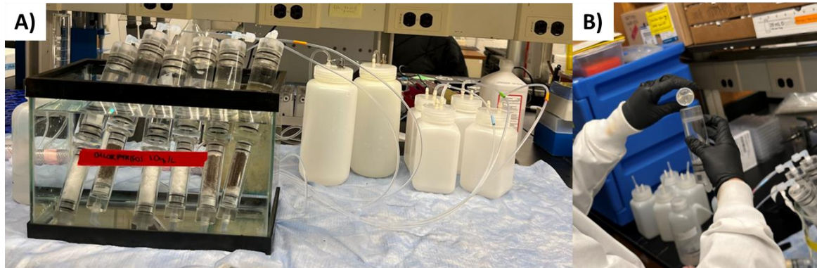
Figure 10: A) Setup for chlorpyrifos exposure, with aquarium tank containing water spiked with chlorpyrifos to a concentration of 1.0 µg/L B) Addition of organisms to iTIE units.
