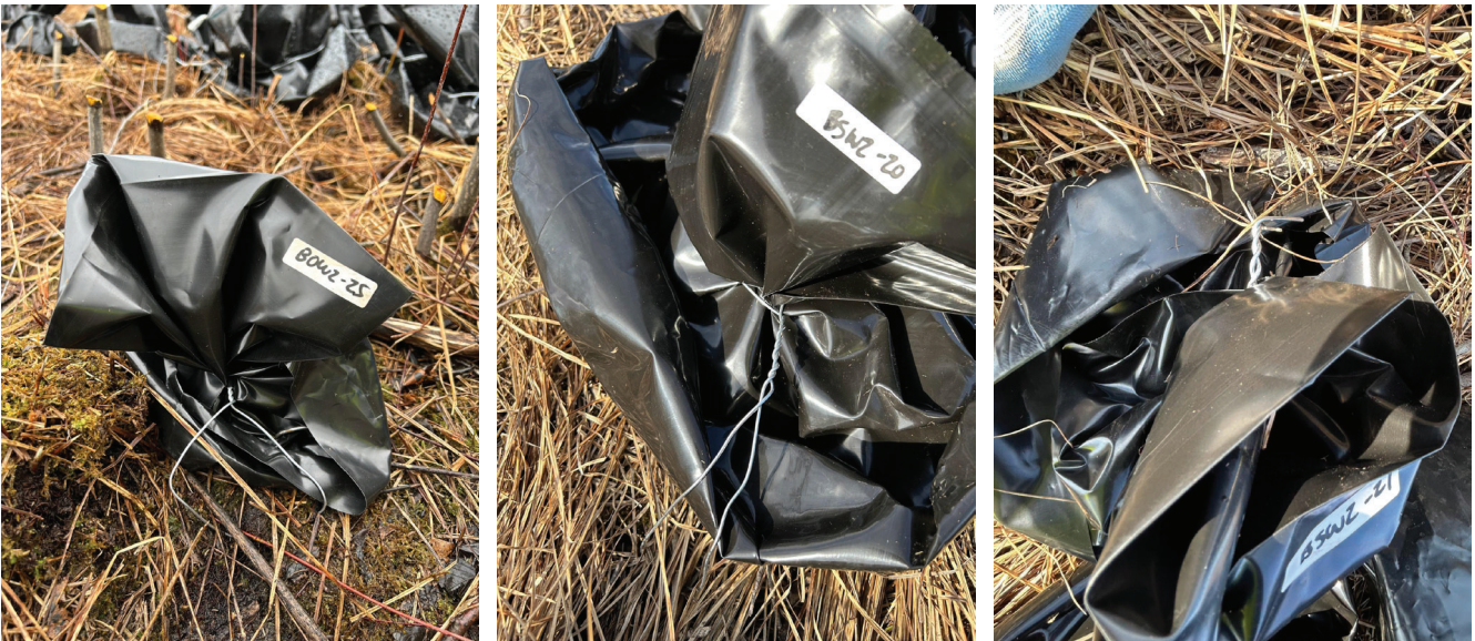
Figure 4.14. 16 gauge galvanized metal wire tied around baggies to secure them to the stem. The left and middle picture exemplifies proper tautness and twisting of the wire with excess length pushed into the ground. The picture on the right exemplifies how shorter excess wire lengths should be bent toward the ground.
