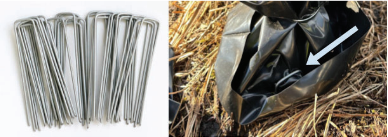
Figure 4.13. A heavy-duty 20 gauge landscaping stake used to secure a buckthorn baggie to the ground.
