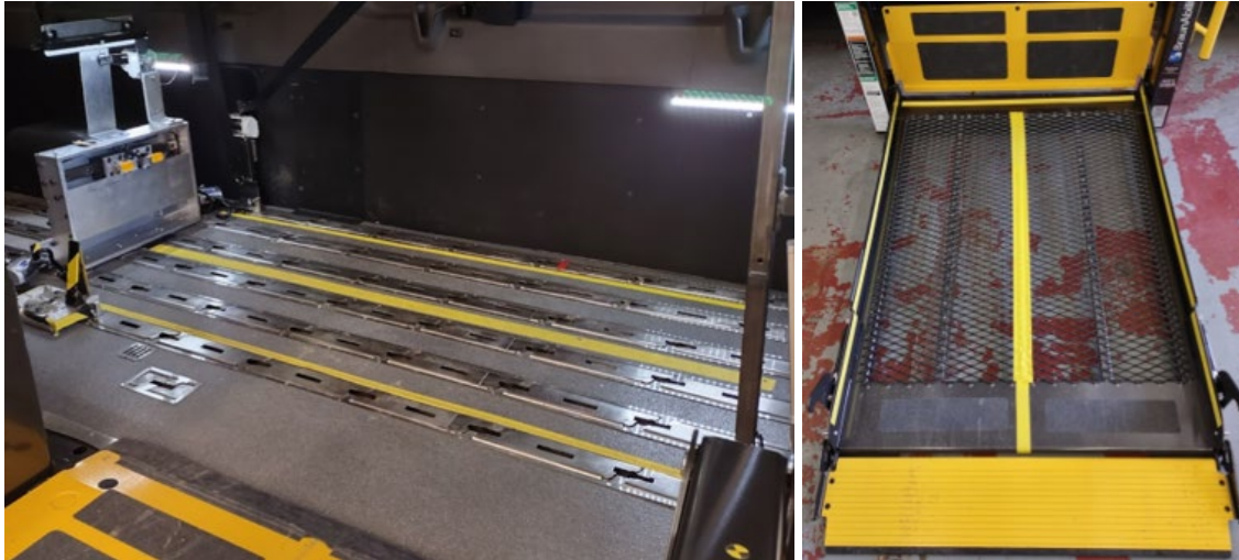
Figure 9. Wheelchair station edges and centerline (left) and ramp centerline (right) marked with contrasting yellow tape.
