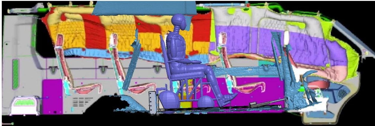
Figure 2. Location of wheelchair station in ~third row relative to vehicle interior geometry.
