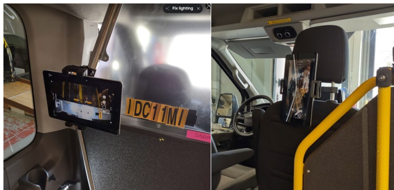
Figure 10. Screen mounted behind driver seat shows top view of UDIG vehicle anchors to assist passenger in aligning and docking their wheelchair (left), and screen mounted on front passenger seat showing path from lift to wheelchair station (right).
