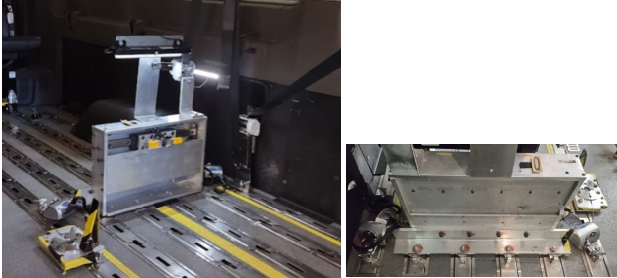
Figure 3. Closeup of UDIG vehicle anchors (left) and how it is secured to track with compatible anchors (right).
