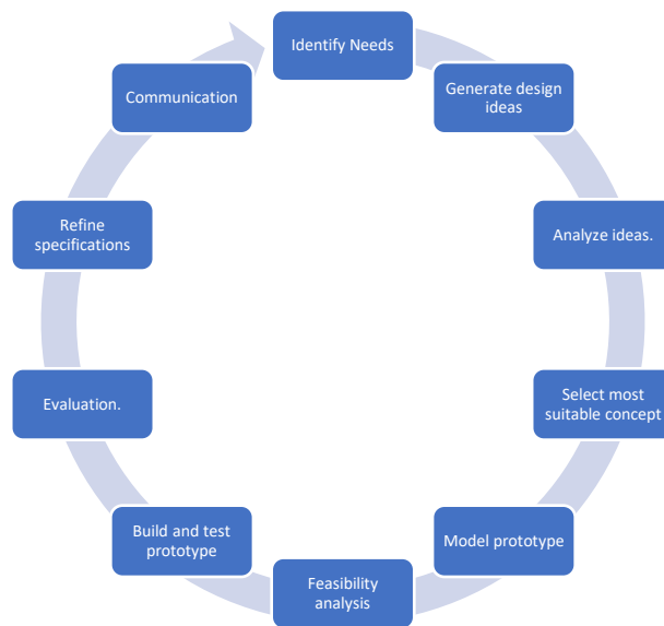
Figure 2-2: The Engineering design Process.
