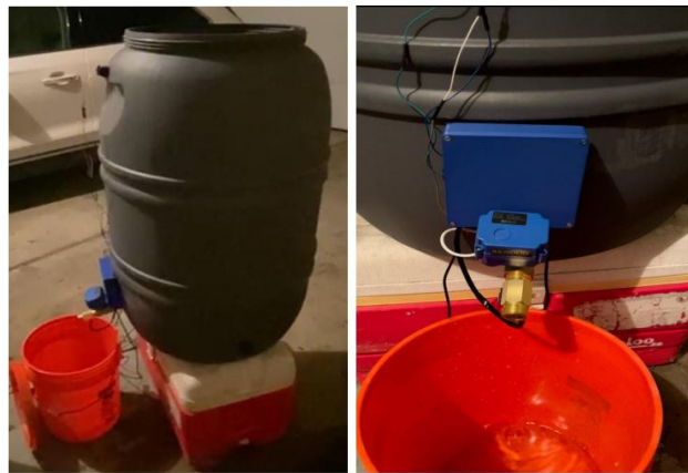
Figure 4 Preliminary prototype SRB developed by the senior design group.
