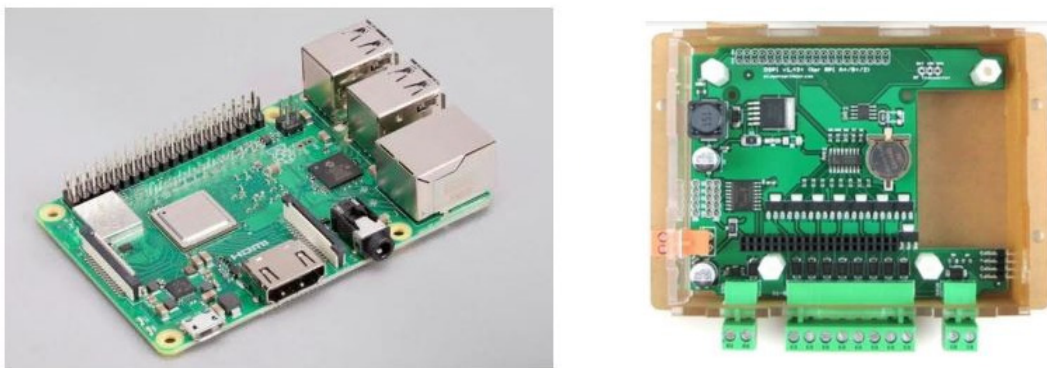
Figure 5 Hardware used for the prototype SRB (Raspberry Pi on left, OpenSprinkler module on right).
