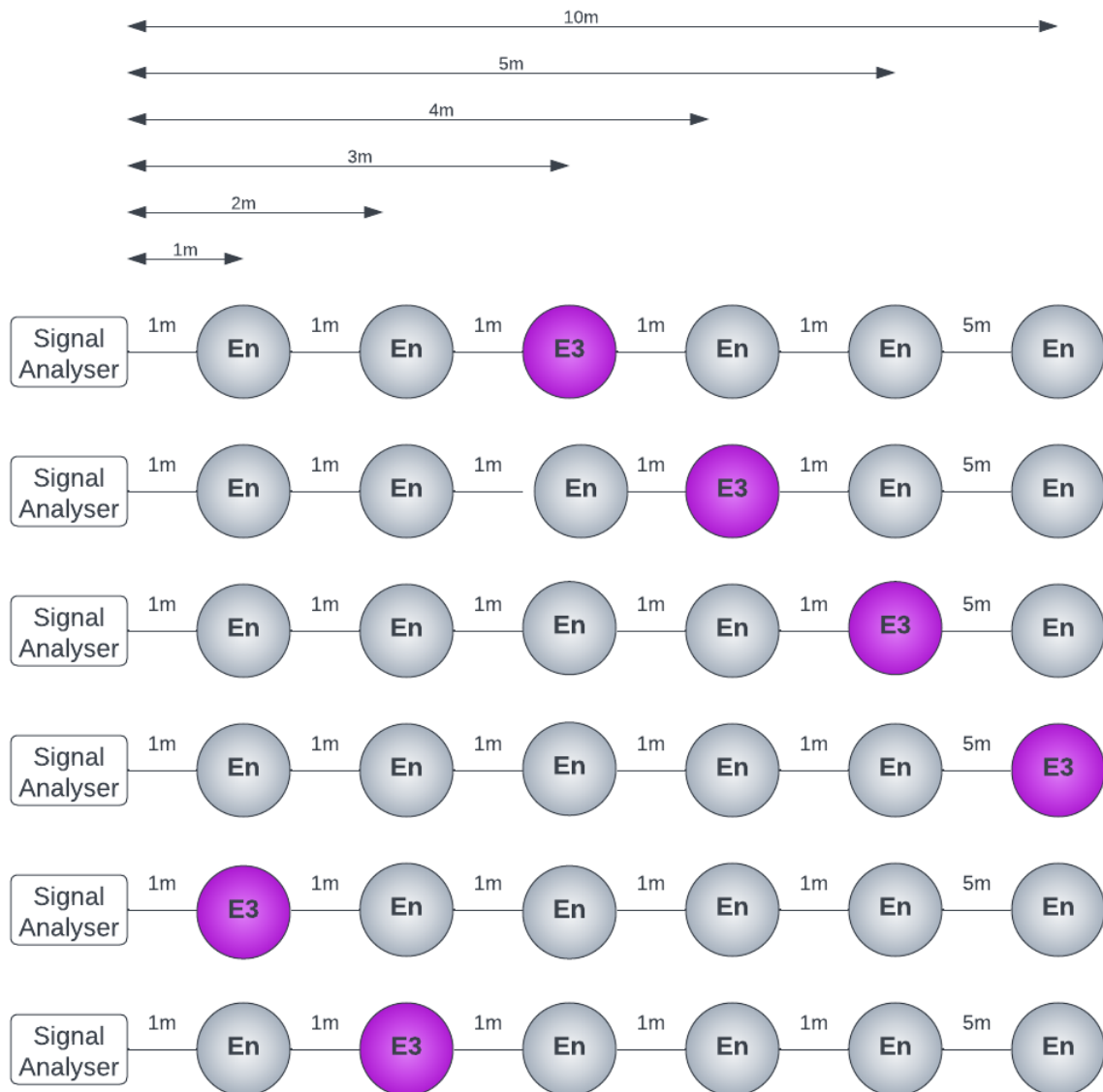
Figure 3.4: Combinations of ECU 3 placement in the CAN with the signal analyser
