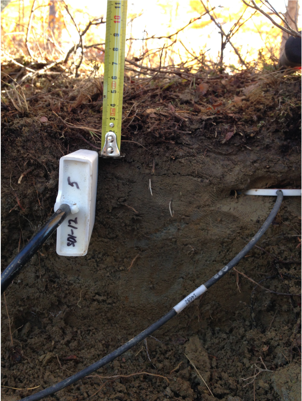
Figure 3.5: Setups for the CS655 water content reflectometer (white box on the left) and the HFP01 heat flux plate (horizontal plate on the right) placed in the mineral soil layer.
