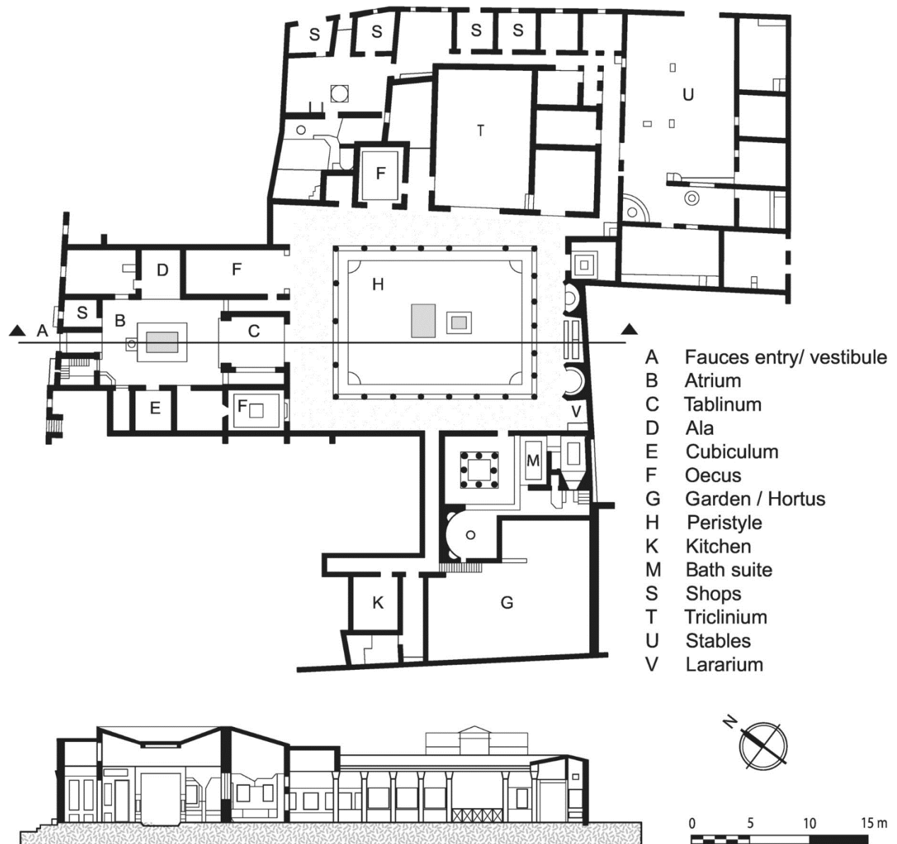
Fig. 5.3. Plan and section of the house of Menander, Pompeii. Note triclinium (room T). (Yegül and Favro 2019, fig. 5.6).
