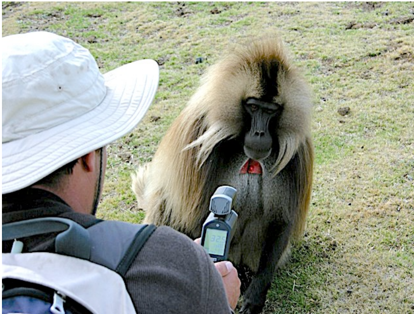
Supplementary Figure 2. Measuring chest patch skin surface temperature. One of the authors (TJB) using a Raytek MX6 PhotoTemp Infrared Thermometer (“temperature gun”) to measure the surface temperature of an adult male’s chest patch. All measurements were taken from 1-2 meters away.
