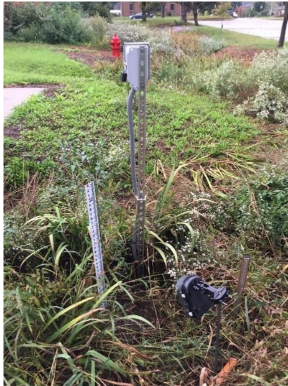
Figure A.1: An example of sensor and camera-measured depths in one GI asset from the validation study completed by an outside consultant.
