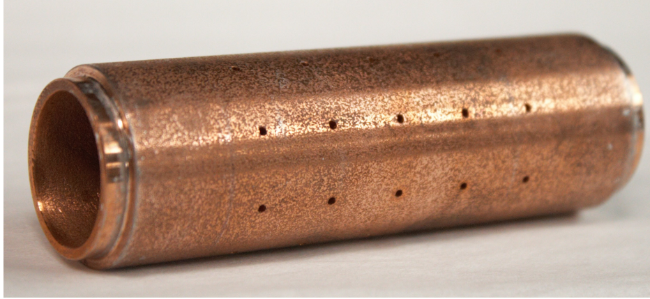
Figure 5.1: Photograph of the SLM-printed outer conductor segment. The total length of this part is 76.2 mm (3.0 in).
