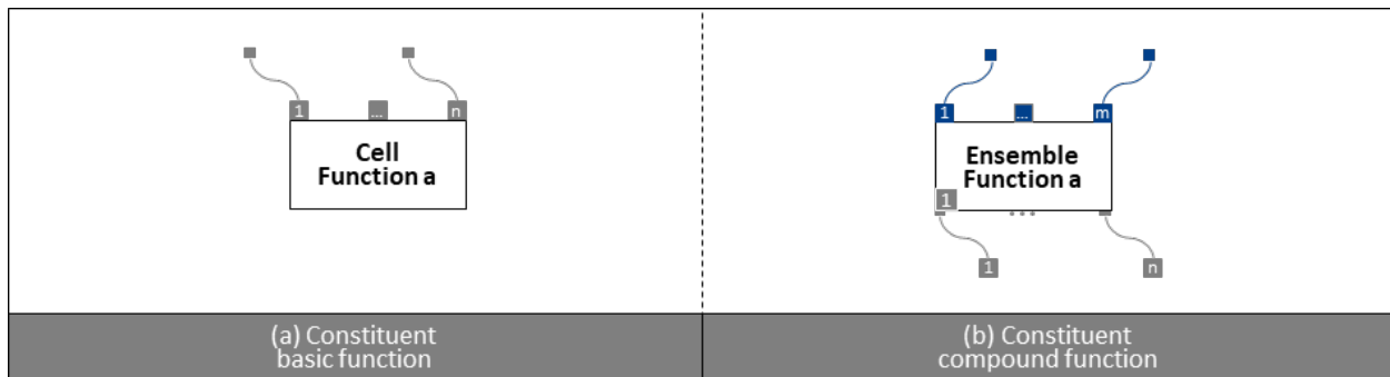
Figure 70. Representations of generic constituent basic (a) and compound (b) functions. a) Cell function a represents constituent basic functions at the cell level, which are directly related to the physical behaviors each cell exhibits once pneumatically activated. b) Ensemble function a represents constituent compound functions, which act as higher-level constituent functional components to form constitutive functional components at the unit level or above.
