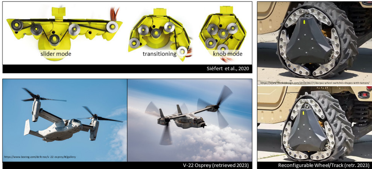
Figure 12. Structurally adaptable multi-mode application examples using conventional electro-mechanically activated component-based approach. Examples include a tangible user interface element that can switch between a rotational knob and a linear slider on demand (top left) [53], the tilt-rotor mechanism of the V-22 Osprey, which allows for vertical takeoff and landing like a helicopter while also enabling high-speed, high-altitude forward flight like an airplane (bottom left) [54]; the reconfigurable wheel-track, which functions as either a wheel or a triangular track in separate modes to achieve high speeds on roads or traverse diverse off-road terrains (right) [4].
