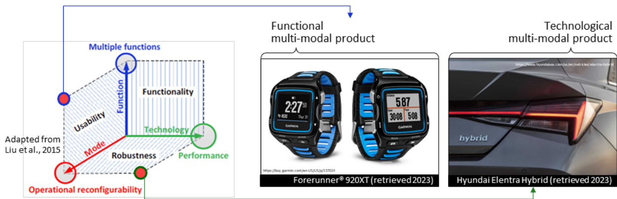
Figure 11. Multi-modal mechatronic design examples. Function-technology-mode paradigm introduced by Liu et al. is shown on the left [47]. Forerunner® 920XT wristwatch (middle) [49] exemplifying function multiplication, and Hyundai Elentra hybrid car (right) [50] exemplifying technology multiplication.
